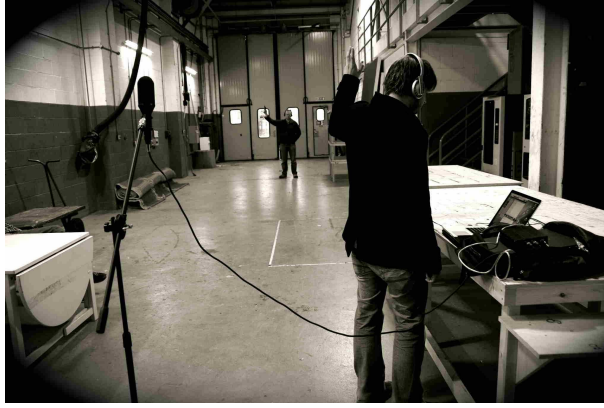
Figure 4: Capturing the B-Format impulse response of a reverberant space
