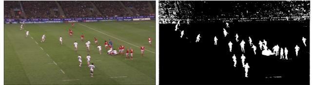
Figure 6. Test sequence 'Rugby', one frame of main camera (left) and key (right).
