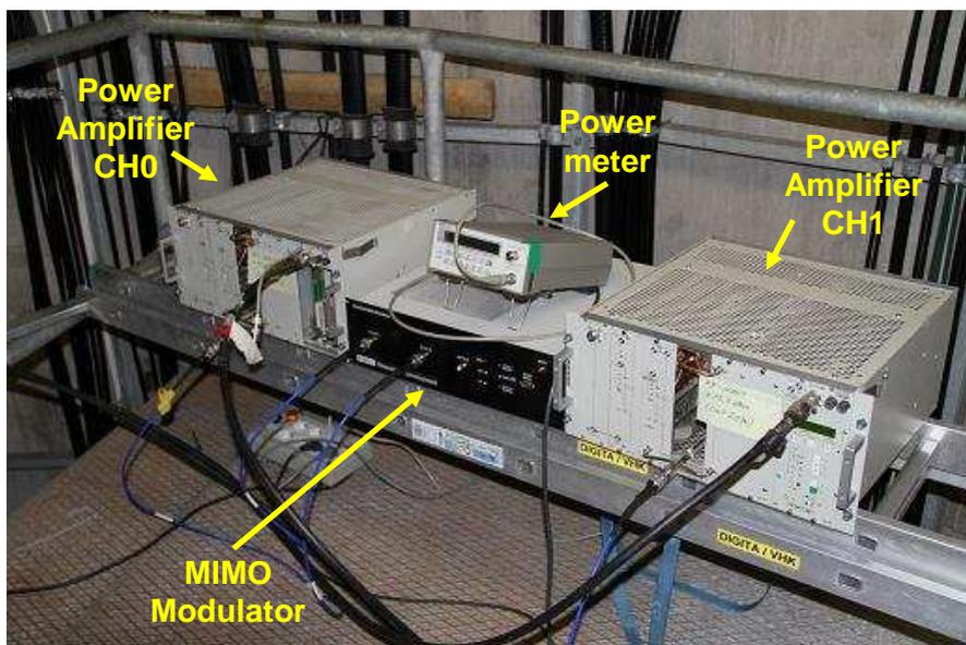
**Figure 4: BBC MIMO Modulator and Power Amplifiers**
