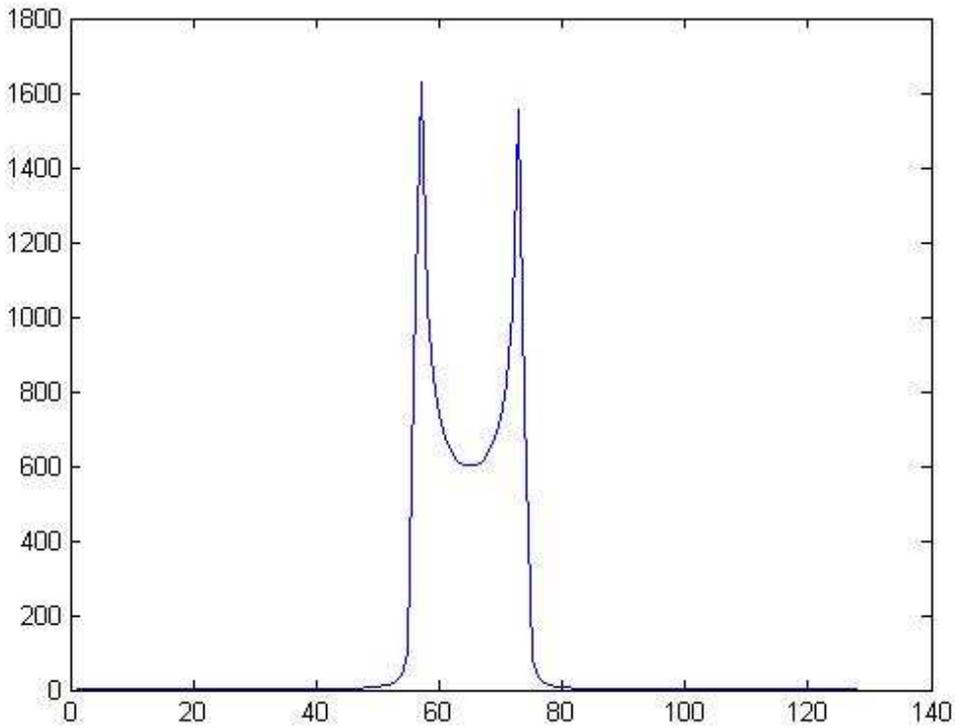
In this model, the Jakes spectrum is specified to be used at a particular tap in conjunction with a fixed frequency offset (pure Doppler) proportional to  $f_d$ . Table 4 below specifies the spectra of each tap.
