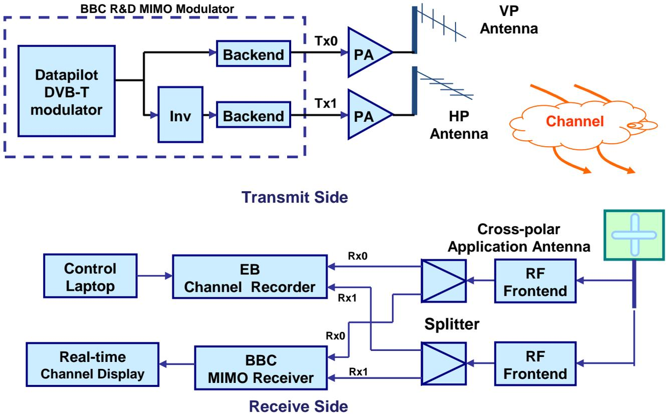
Figure 2: Block diagram of transmit and receive side
