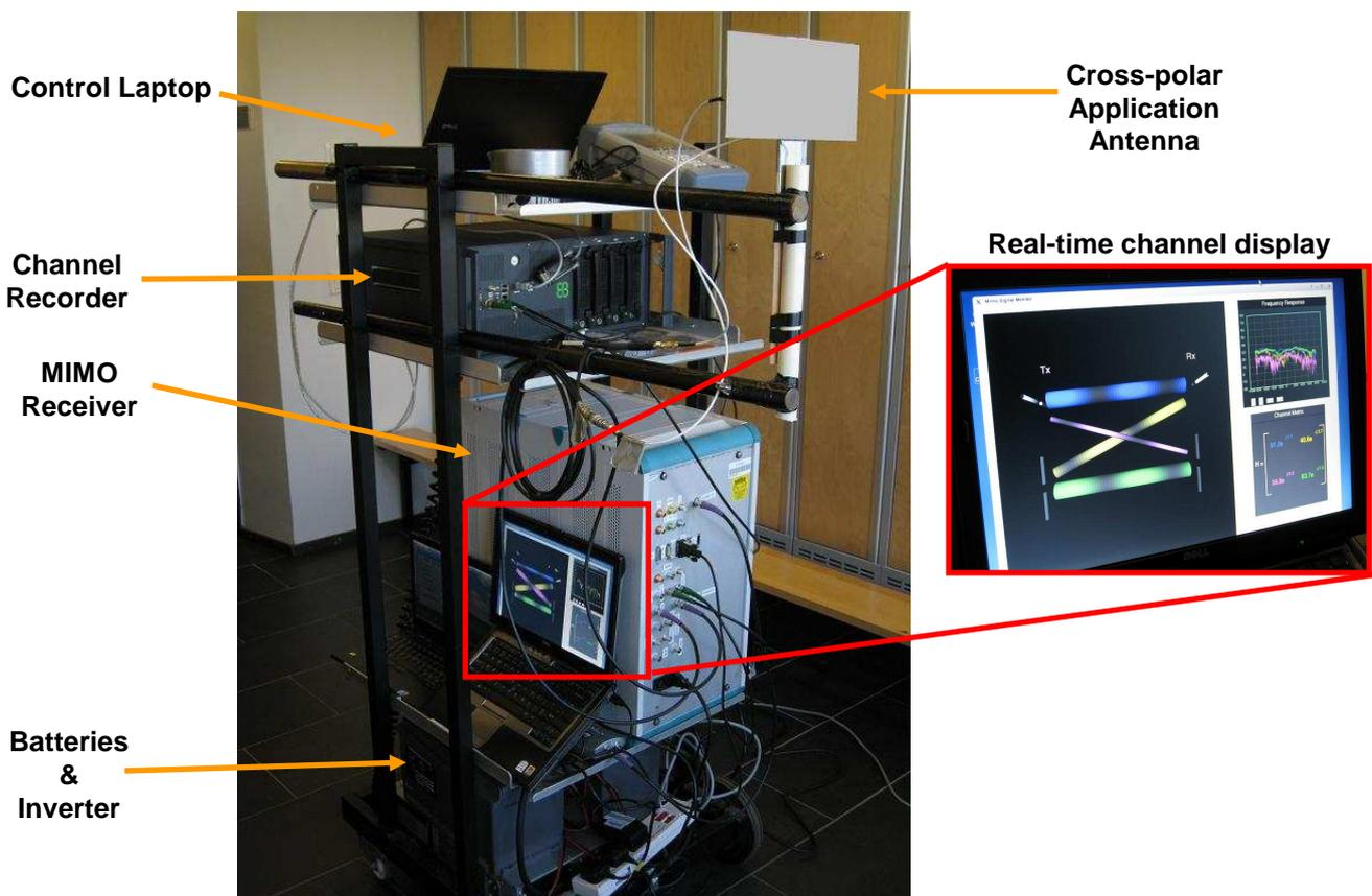
**Figure 5: Portable receiving station**
