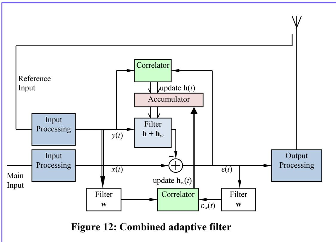
However, the additional adaptive filter  $\mathbf{h}_w$  can be constrained to reduce noise even further. Instead of trying to estimate individual taps of  $\mathbf{h}_w$ , just two coefficients can be used, one for the lower and one for the upper out-of-band region. This is done by combining the above method of figure 12 with the transform-LMS algorithm. The error can be redefined as:
