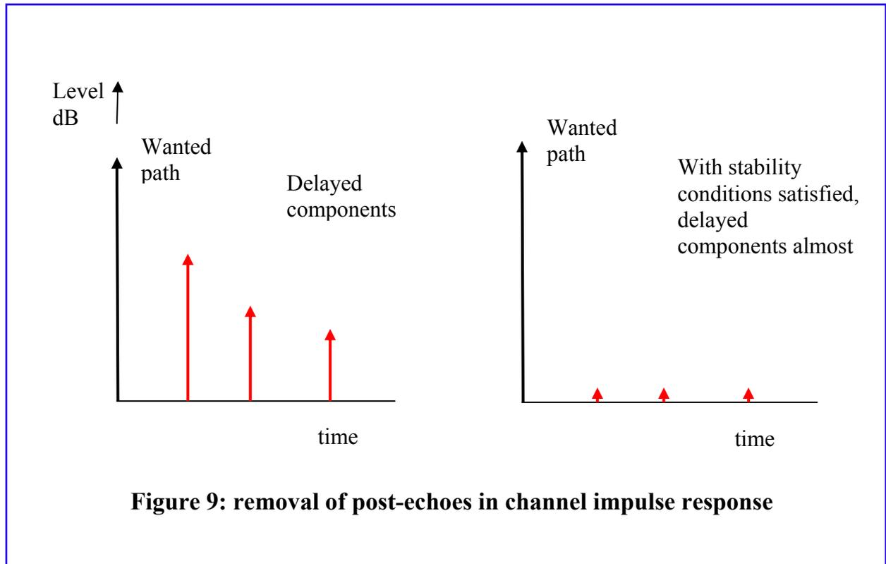
**Figure 9: removal of post-echoes in channel impulse response**
