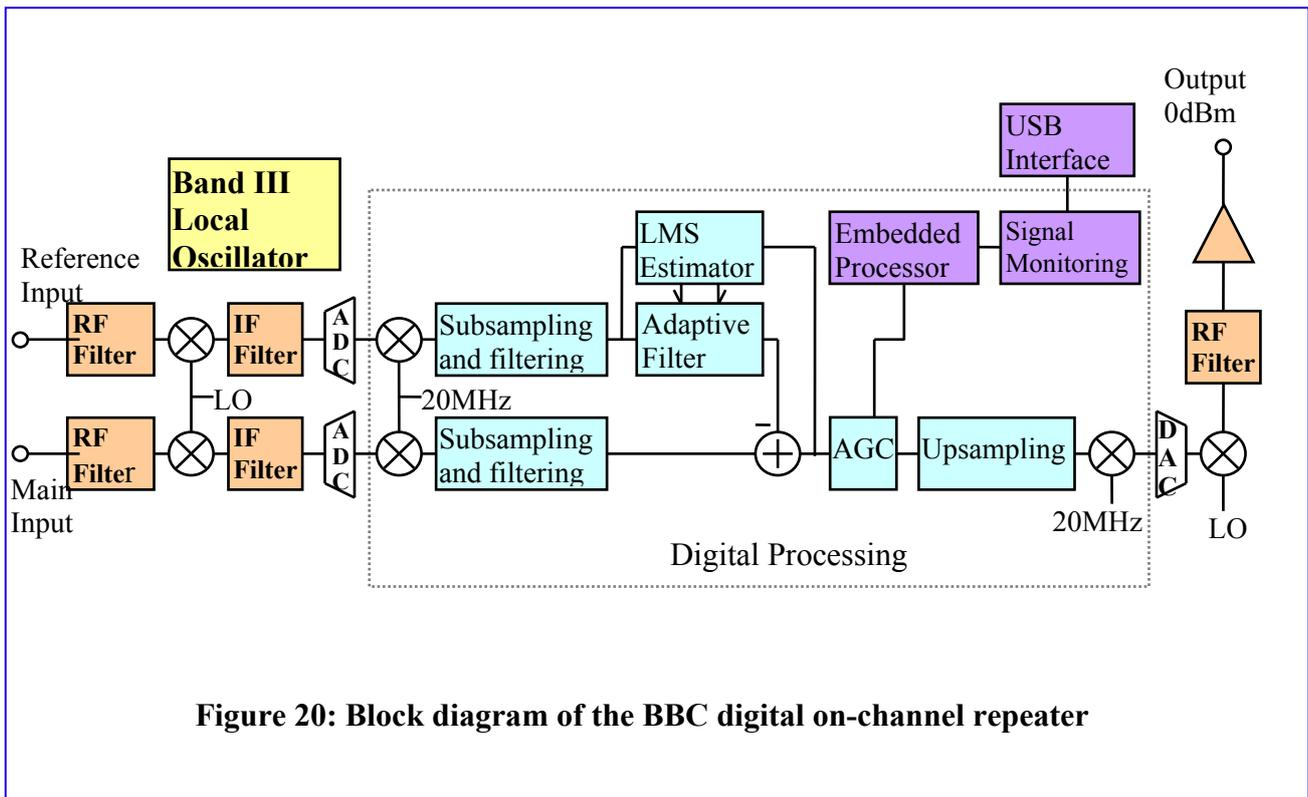
**Figure 20: Block diagram of the BBC digital on-channel repeater**
