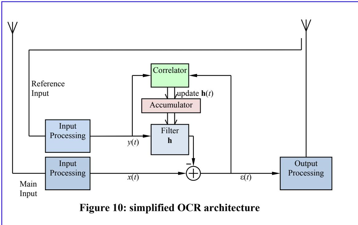
**Figure 10: simplified OCR architecture**
