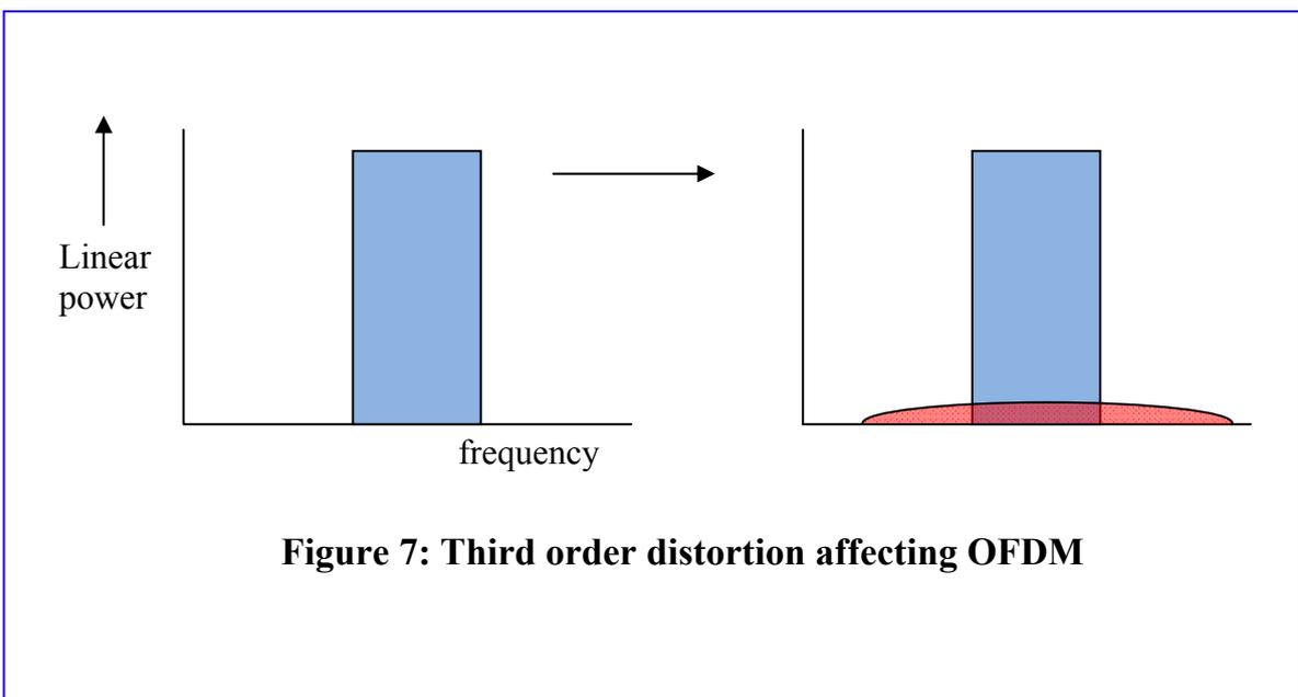
The distorted spectrum is made up of the sum of the original signal, and a term which essentially results from a double convolution of the signal PSD with itself, producing a triangular PSD after the first convolution and a softened inverted bowl-shape from the second convolution.
