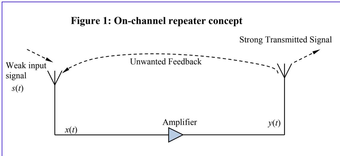
**Figure 1: On-channel repeater concept**
