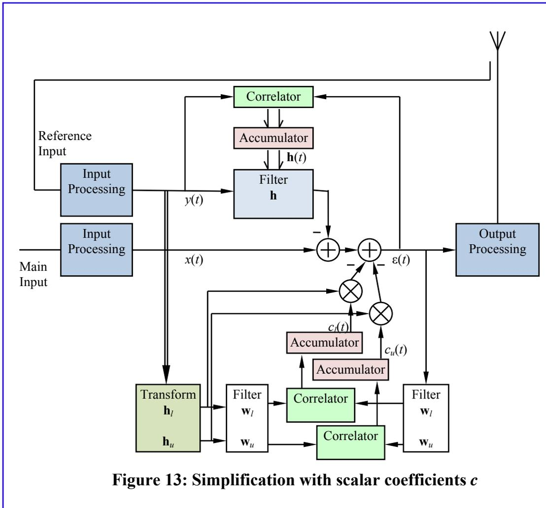
**Figure 13: Simplification with scalar coefficients  $c$**
