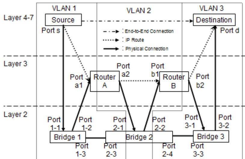
Figure 7: Cross-VLAN Path Tracing
