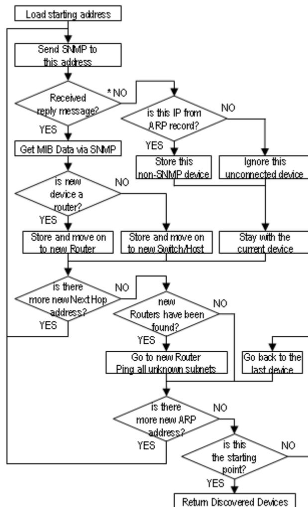
Figure 5: Device Discovery Algorithm
