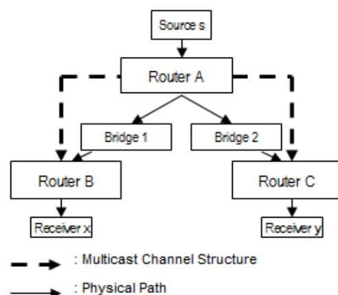
Figure 8: Physical Path for Multicast Traffic
