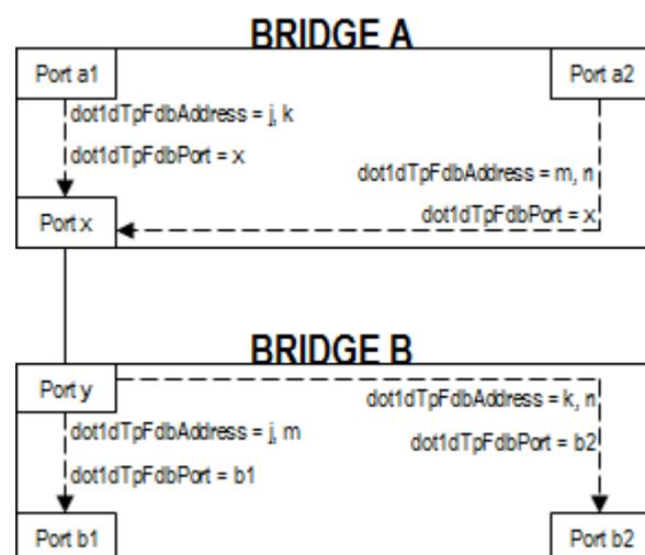
Figure 6: Determining an L2-L2 Connection
