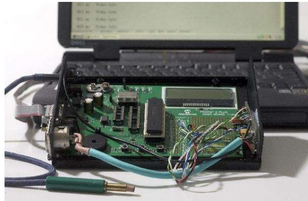
Figure 5 Prototype A/V measurement system, with laptop PC logging the measurements
