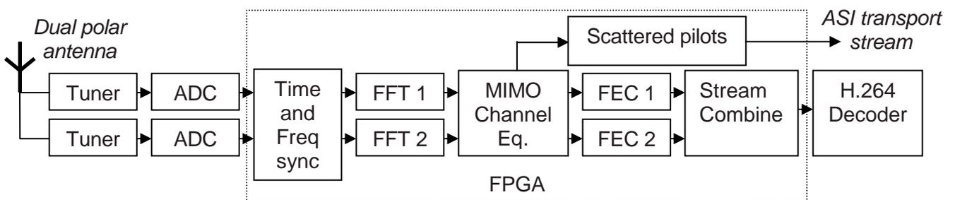
**Figure 1 - Receiver architecture**
