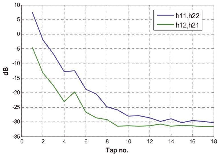
Figure 5 - Typical Portable Power Delay Profile
