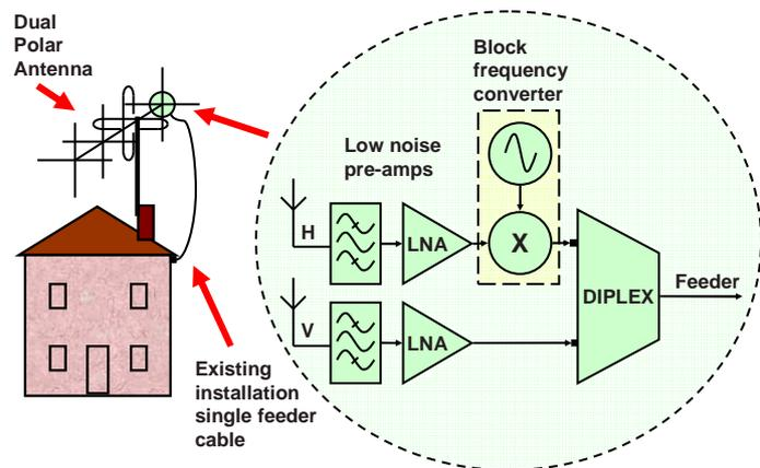
**Figure 7 - Block frequency conversion allows reuse of existing single feeder cable**
