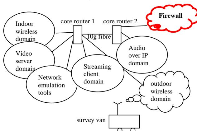
Figure 1. BBC Research video / audio over IP test network bed
