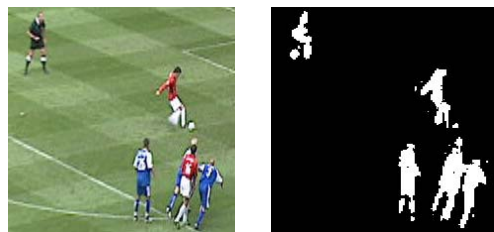
Fig. 4. Test image (left), results of fast green segmentation (right).
