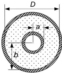
If the radius of the outer surface of the inner conductor is  $a$ , the radius of the inner surface of the outer conductor is  $b$ , and a voltage  $V$  (shorthand for a potential difference,  $\Delta V$ ) is applied between the conductors:
