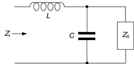
$$\begin{aligned} Z_i &= j\omega L + \frac{Z_0(1/j\omega C)}{Z_0 + 1/j\omega C} = j\omega L + \frac{Z_0}{1 + j\omega Z_0 C} = \frac{Z_0(1 - \omega^2 LC) + j\omega L}{1 + j\omega Z_0 C} \\ &= \frac{Z_0(1 - \omega^2 LC) + j\omega L}{1 + j\omega Z_0 C} \cdot \frac{1 - j\omega Z_0 C}{1 - j\omega Z_0 C} = \frac{Z_0(1 - \omega^2 LC) + \omega^2 Z_0 LC + j\omega L - j\omega Z_0^2 C(1 - \omega^2 LC)}{1 + \omega^2 Z_0^2 C^2} \end{aligned}$$
