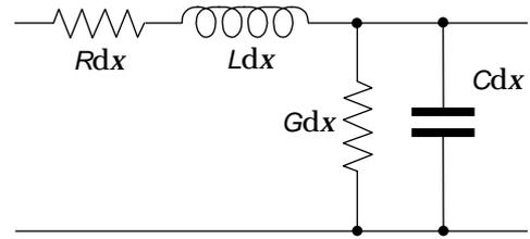
The full expression for the characteristic impedance of a transmission line in the presence of loss becomes:
