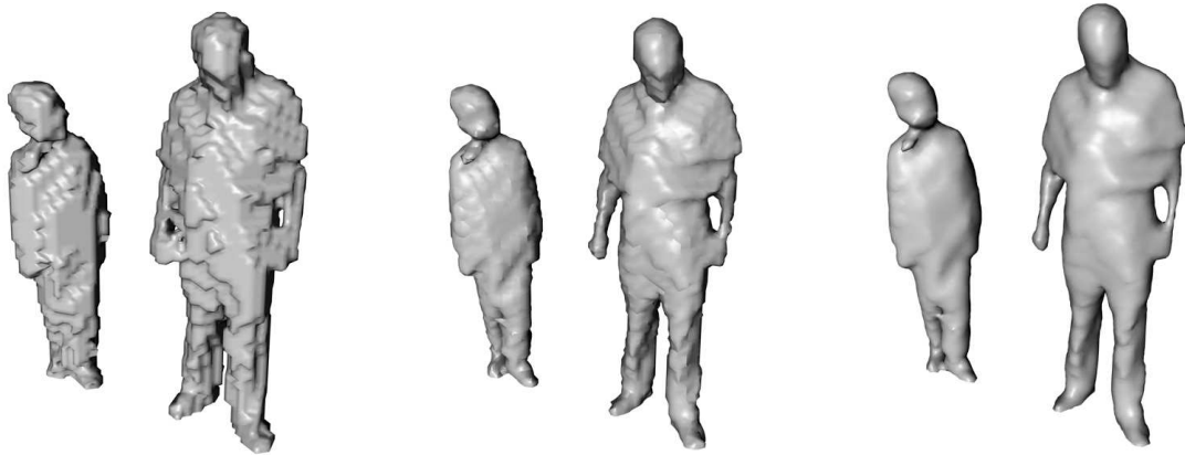
Figure 5. Results of the visual hull computation using standard octree (left), super-sampling (middle) and additional smoothing (right).
