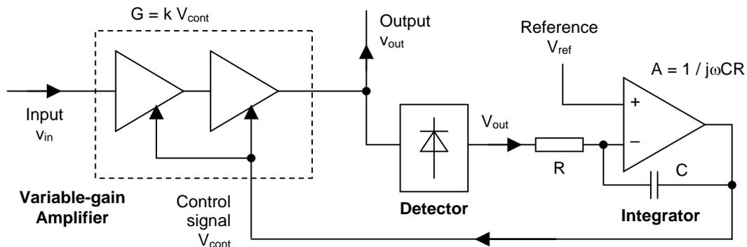
**Figure 2.1:** A Single-loop AGC System
