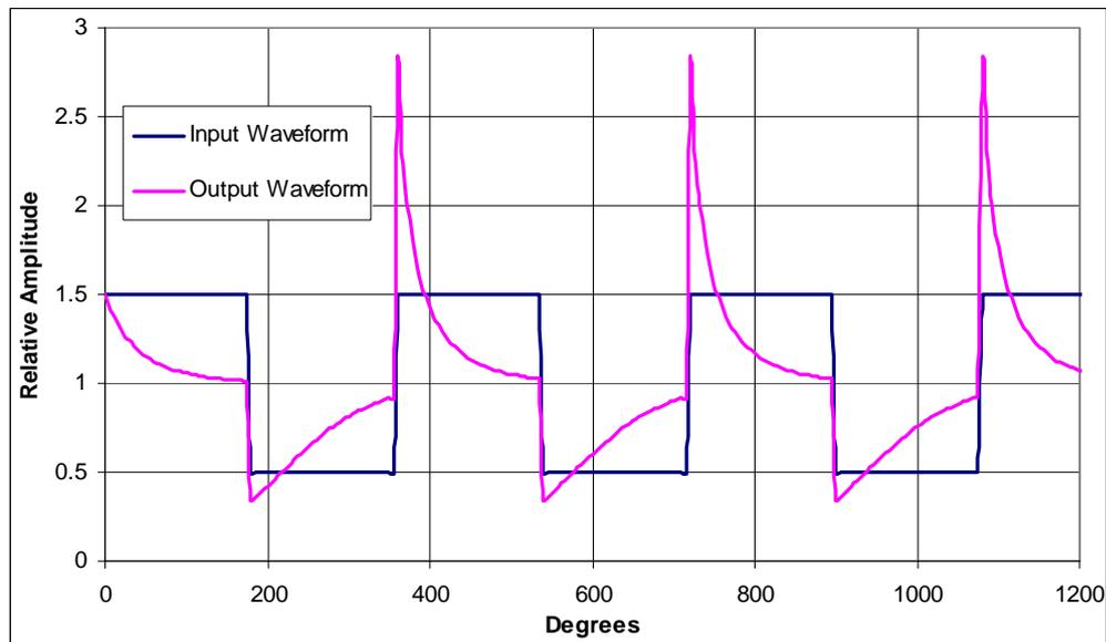
**Figure 7.3:** A Simulation of the AGC Loop Transient Response
