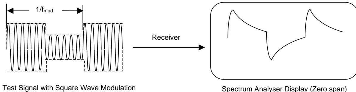
**Figure 5.1:** Checking the AGC Loop Transient Response
