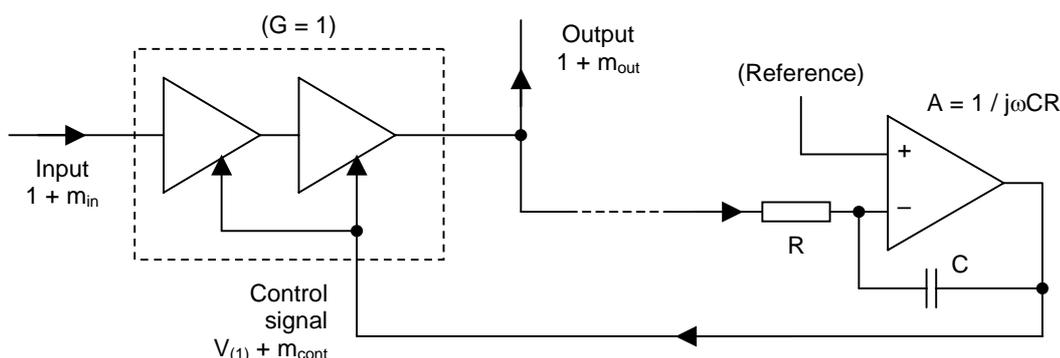
**Figure 2.2:** The Single-loop AGC System with Varying Input
