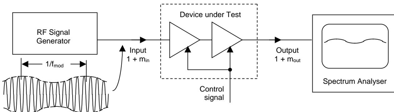
**Figure 4.1:** Set-up for Checking the AGC Loop Bandwidth
