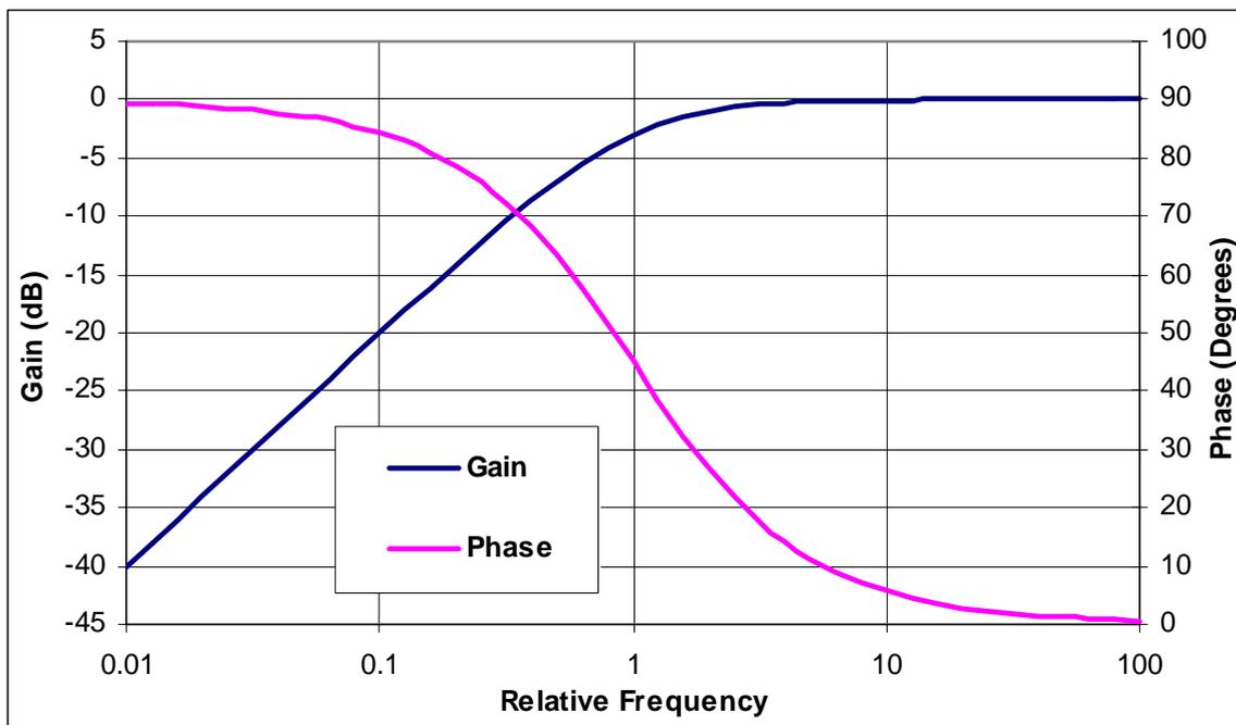
**Figure 2.3:** The Response of the AGC System to Input Variations
