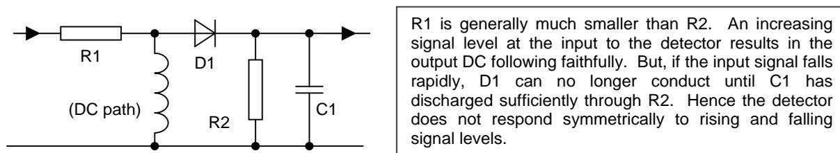
**Figure 6.1:** A Diode Detector Circuit
