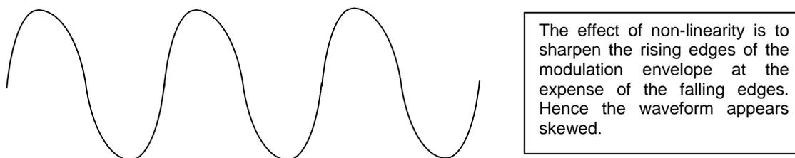
**Figure 6.2:** The Distorted Modulation Envelope
