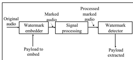
Figure 1 Simplified audio watermarking system
