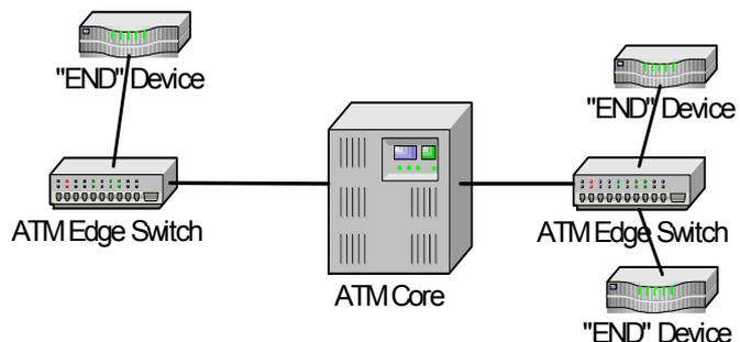
Figure 5: Simple ATM structure.
