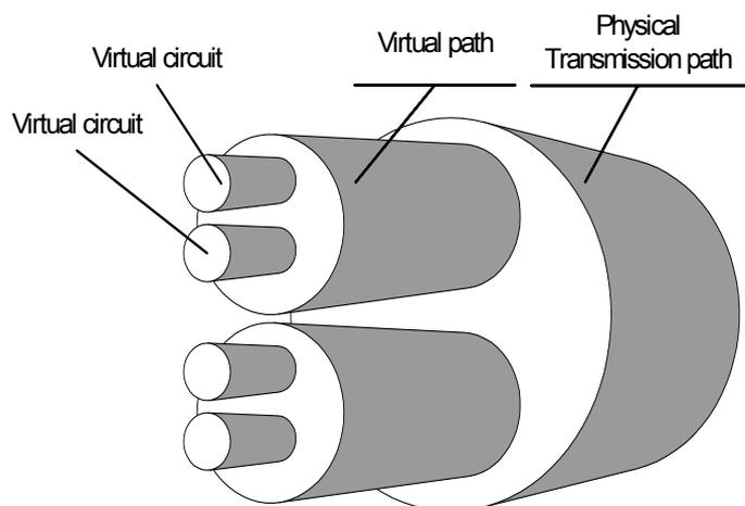
Figure 4: A pictorial representation of the ATM transport structure.
