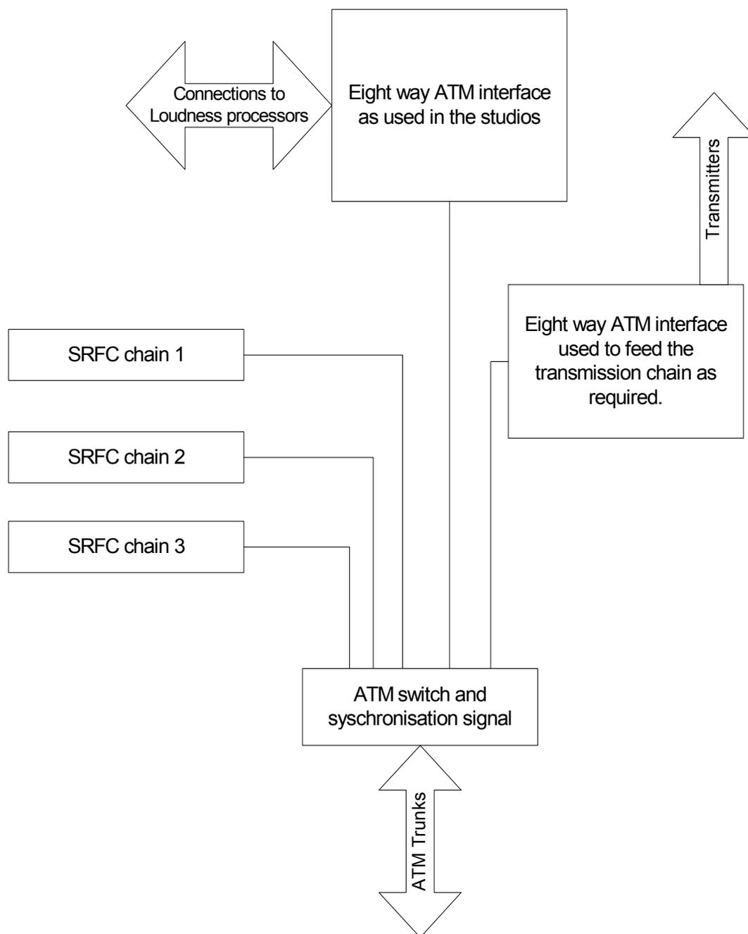
Figure 8: The transmission chains
