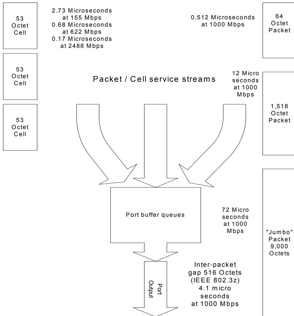
Figure 6: Packet / Cell serialisation
