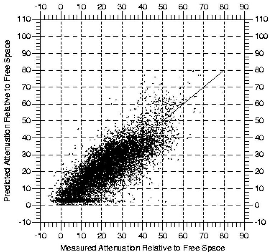
Figure 6 - The excess loss of the UKPM model assuming 50 m resolution
