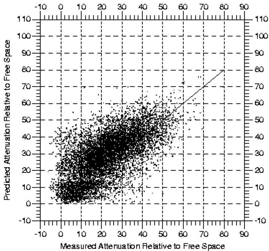
Figure 5 - The excess Loss for the BBC model assuming 500 m resolution
