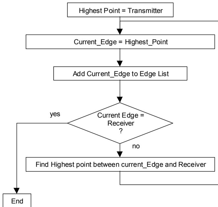
Figure 4 - Description of the edge detection algorithm
