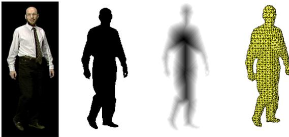
Figure 5: Shape from one silhouette. a) camera image, b) object mask, c) 2D distance function, d) 3D mesh.
