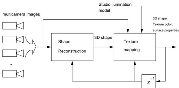
Figure 6: Generation of dynamic 3D models of actors in ORIGAMI
