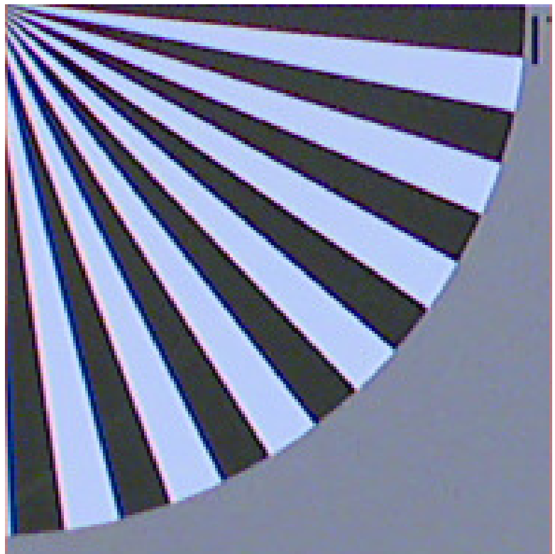
Figure 7 lens aberration, EX1
