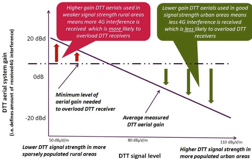
Figure 2 Antenna System Gain versus DTT signal level
