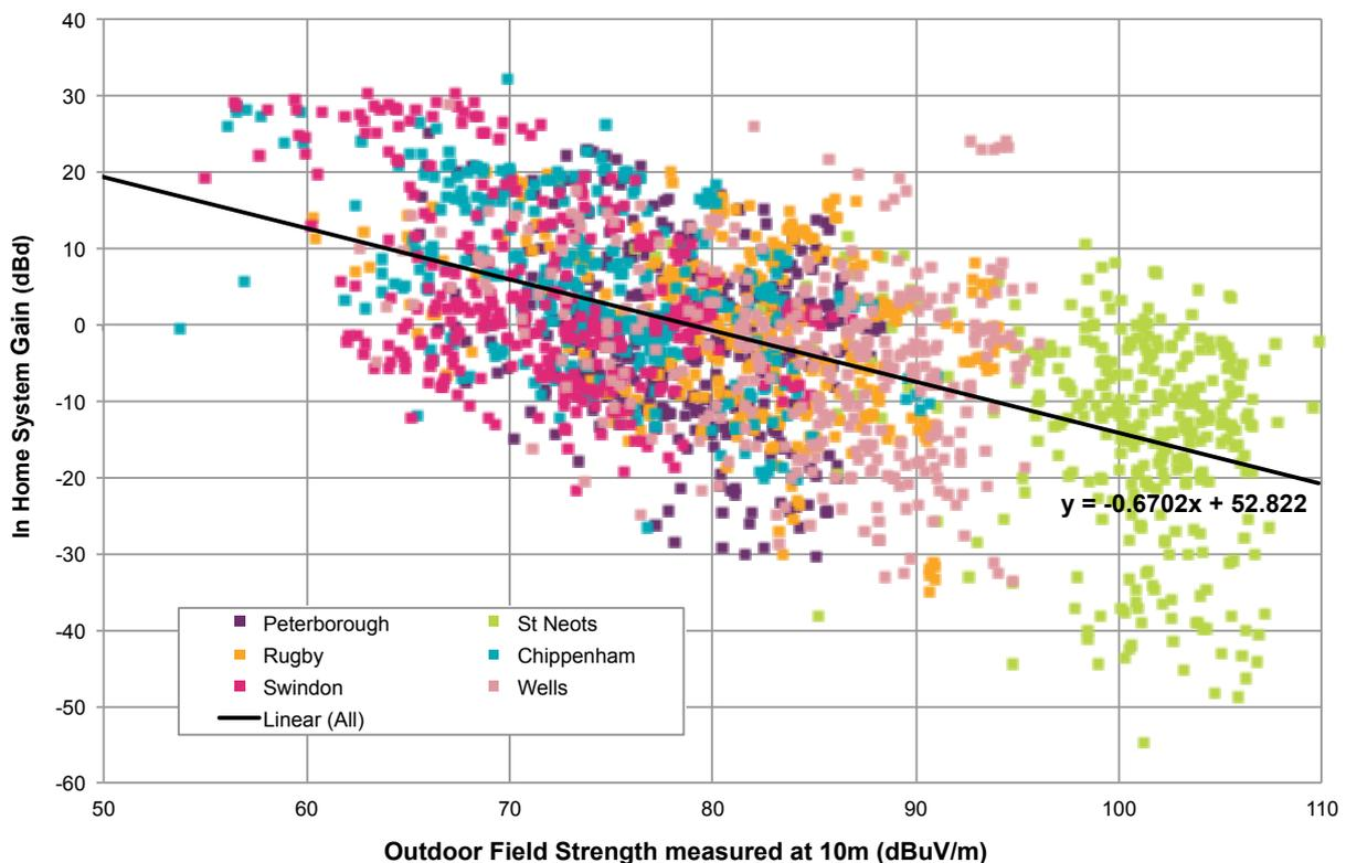
Chart 1 - Measured system gain against measured outdoor DTT field strength
