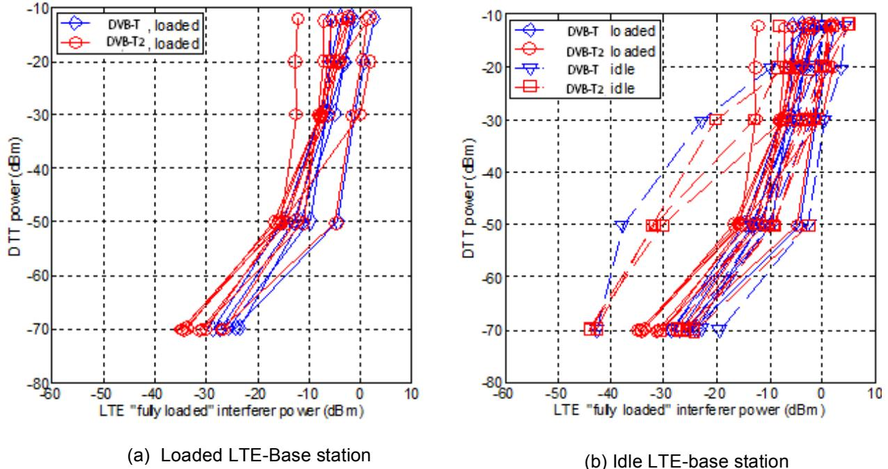
Figure 3: Carrier vs Interferer characteristics for 5 DVB-T DVB-T2 receivers for LTE at 796MHz, DTT at 786 MHz showing impact of base station load
