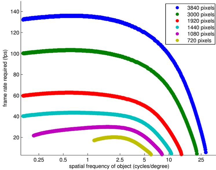
Figure 5: Minimum frame rate required for each point along the “equal blur” contours, for selected spatial resolutions at a viewing distance of  $1.5H$ . The contour marked in black in figure 4 is for 3840 horizontal pixels, and corresponds to the dark blue (uppermost) curve here. The peak of each curve is taken as the required frame rate to match that spatial resolution.
