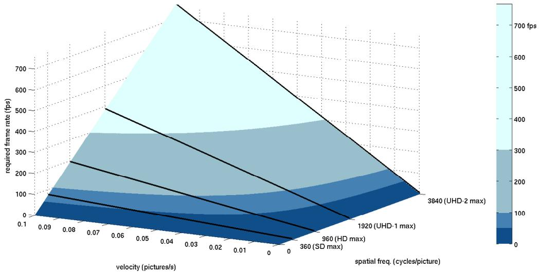
Figure 8: Frame rates required to represent a range of horizontal frequencies moving at different velocities, without aliasing. The four thick lines indicate the maximum spatial frequency (half the number of horizontal pixels) for some common spatial formats.
