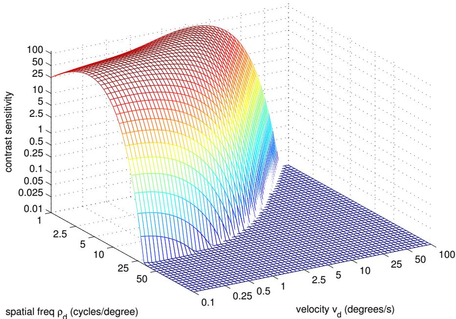
Figure 1: Kelly-Daly model of the human contrast sensitivity function, as described by Laird et al. [2006].
