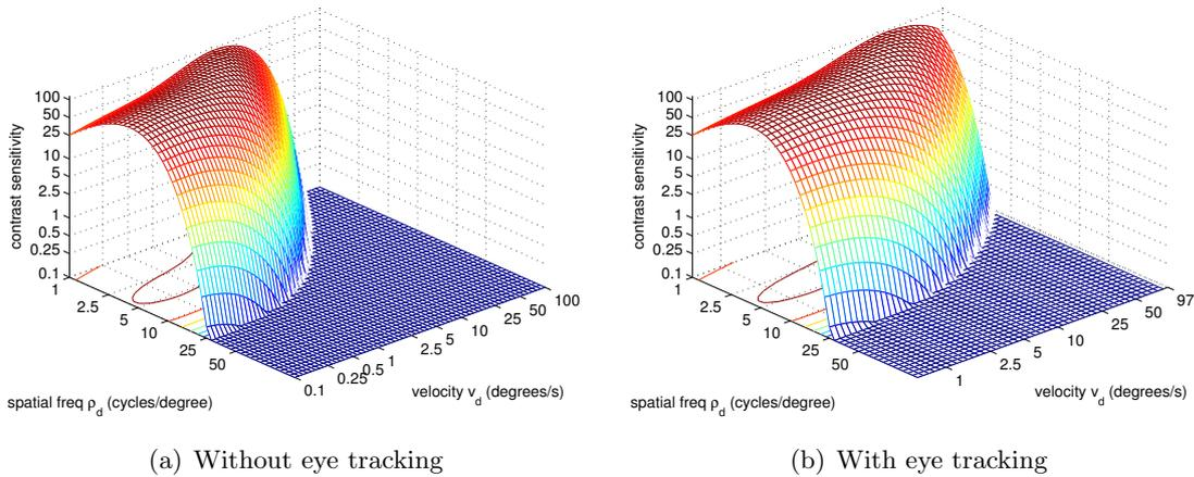
Figure 7: Comparison of contrast sensitivity function without and with modification to include a model of eye tracking.
