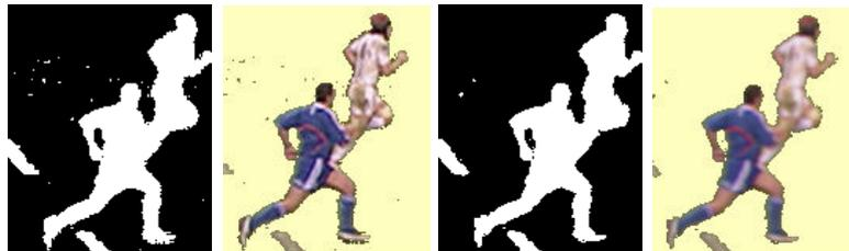
**Fig. 4** Detail of segmented broadcast picture before compensation for aperture correction (left) and after compensation (right)
