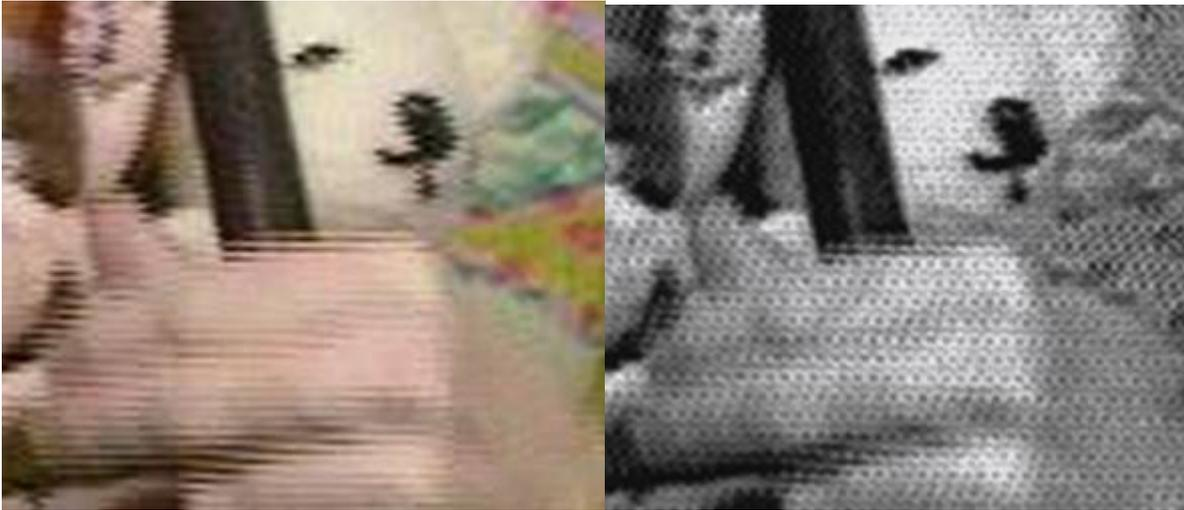
Figure 11 - original colour video recording and 'chroma dots' in a non-filtered B&W telerecording.
