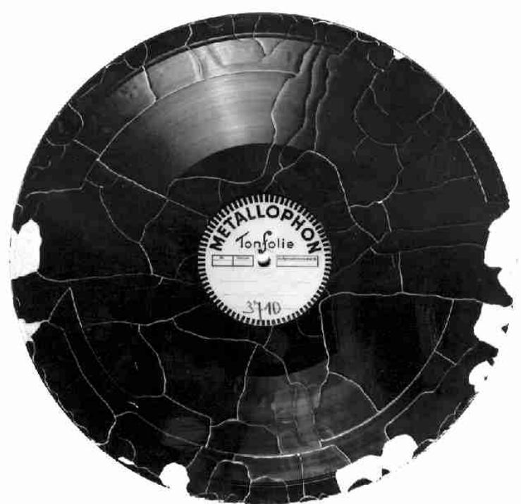
Figure 6 - A damaged acetate disc.
