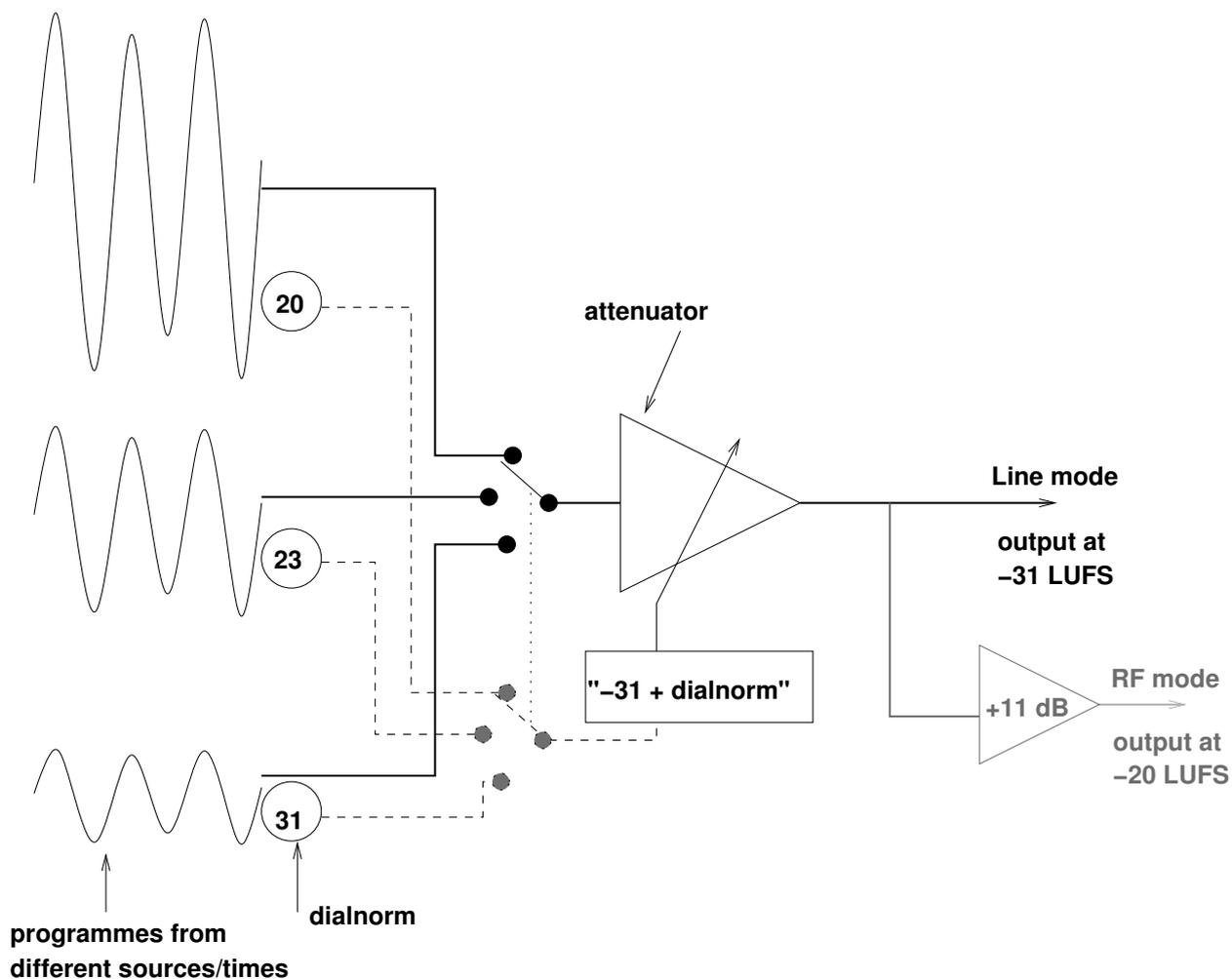
Figure 2: Use of “dialnorm” in Dolby Digital decoder to normalise to -31 LUFS
