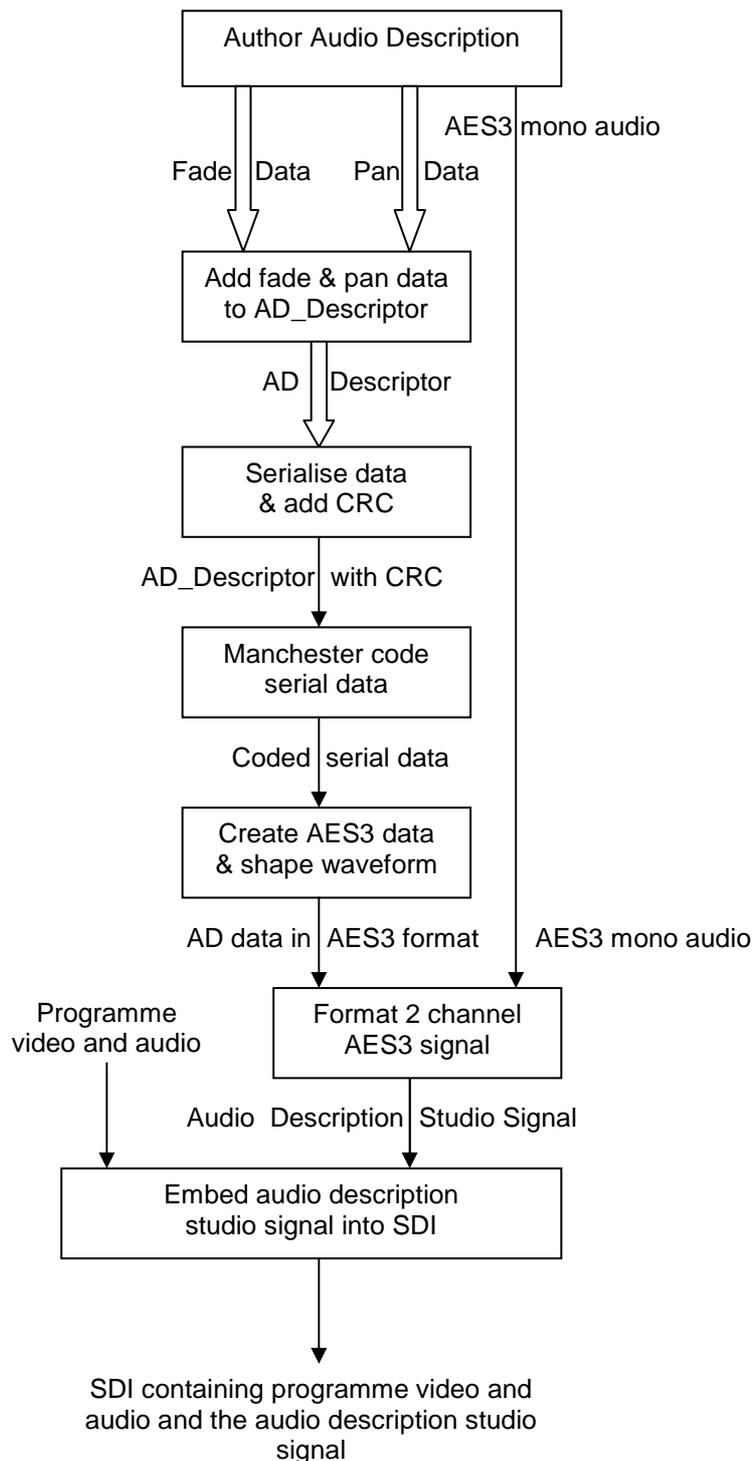
Figure 1. Flowchart showing the generation of the audio description studio signal
