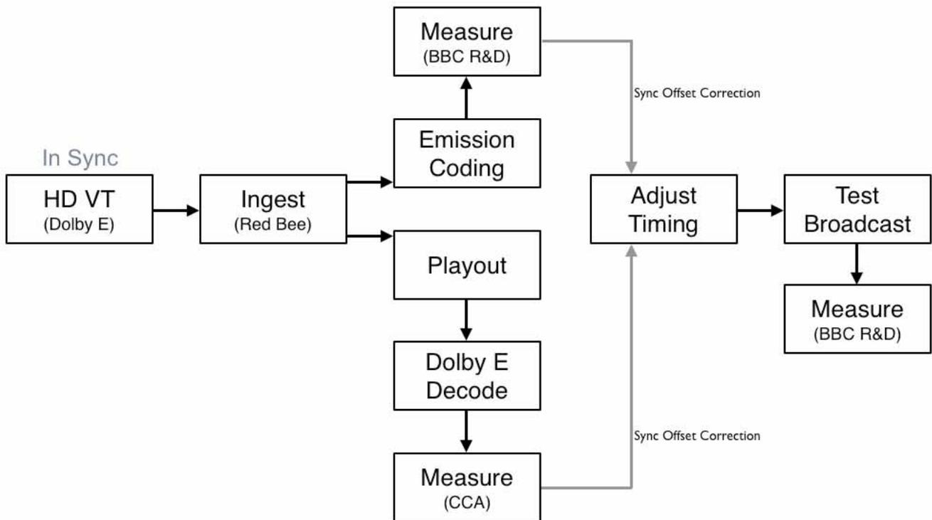
Figure 13 - Measuring sync in the broadcast chain
