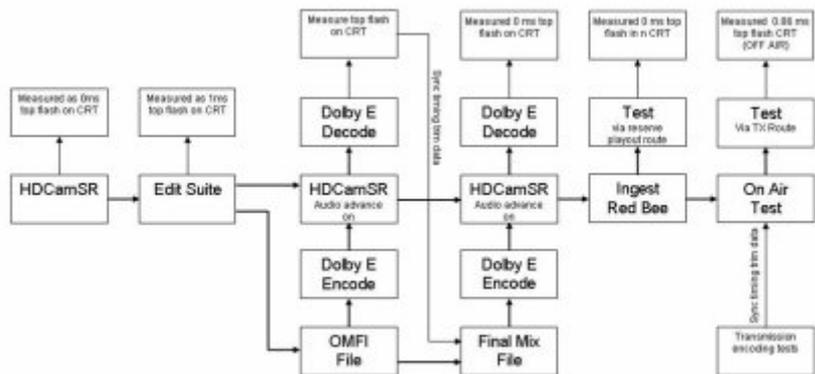
The effect of AV sync has been measured and tested quite extensively by the international broadcast standards bodies and we usually work to a tolerance of +20ms to -40ms (+half to - 1 frame) for a programme delivered to the BBC. This tolerance has been well tested in SD but there has not been enough work done to see if it's still OK in HD. To make sure there were no major surprises we have tightened the delivery specification to +10ms to -20ms while we do more tests.
