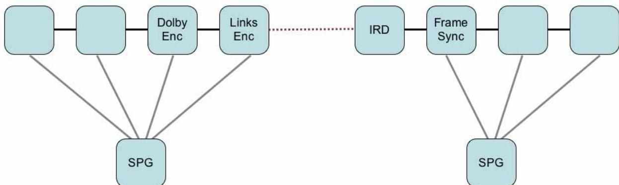
Figure 5 - Contribution link timing, with an IRD locked to incoming video
