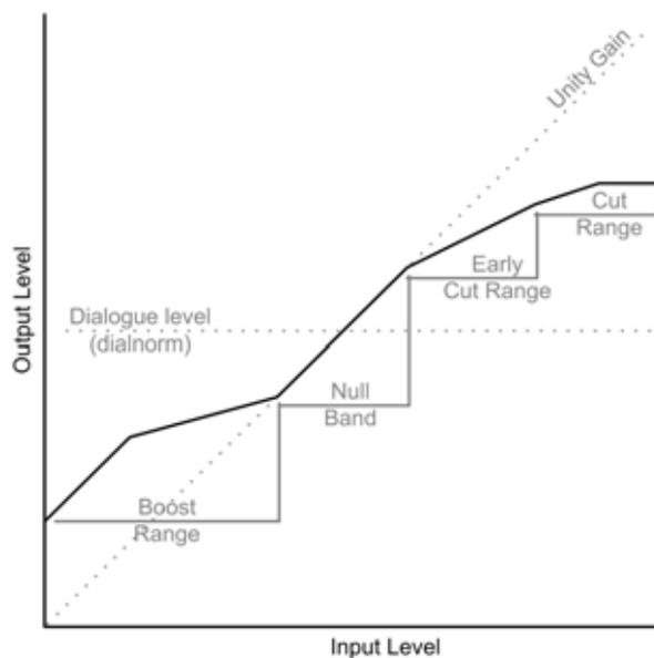
Figure 14 - Dynamic Range Control in a Dolby Digital decoder
