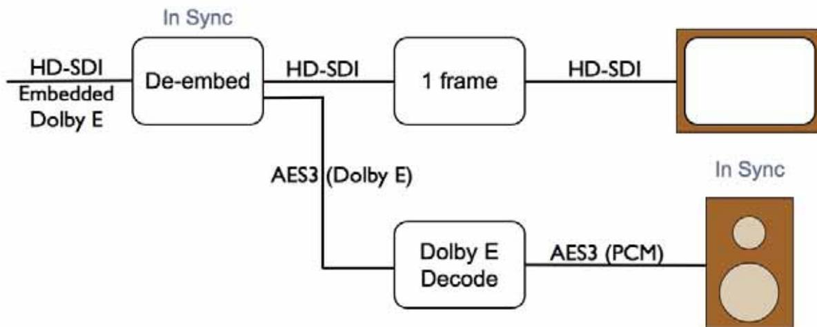
Figure 8 - The BBC's chosen delivery and delay solution for Dolby E
