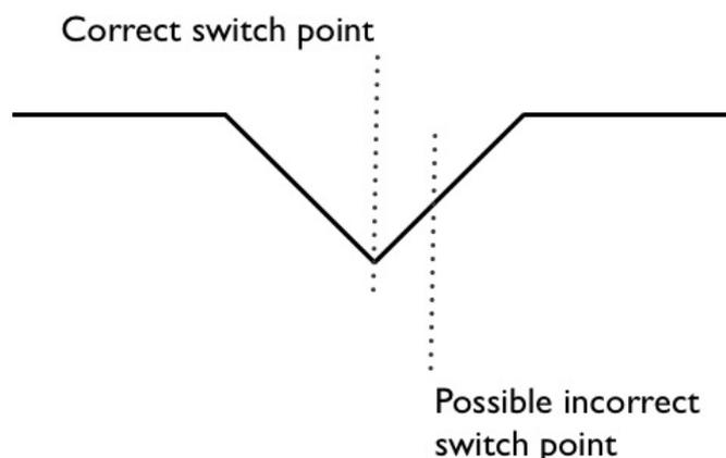
Figure 7 - The effects of decoding latency on V-fades
