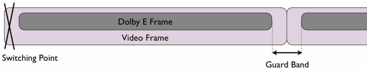
Figure 3 - Simplified Dolby E timing (not to scale)
