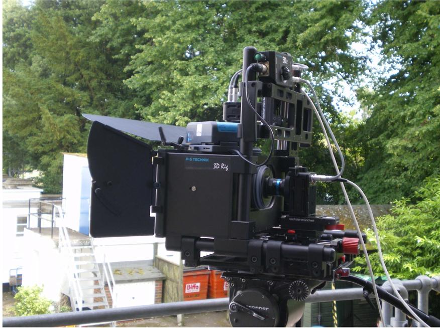
Figure 1: A photograph of the P+S Technik mirror rig, shown here equipped with Silicon Imaging SI-2K Mini camera heads (right and, partially concealed, on top). Also visible are a P+S Technik 3d sync box (mounted top right) powered by a camera battery (resting on top of the rig, in front of the top camera), which provides timing information to synchronise the cameras.
