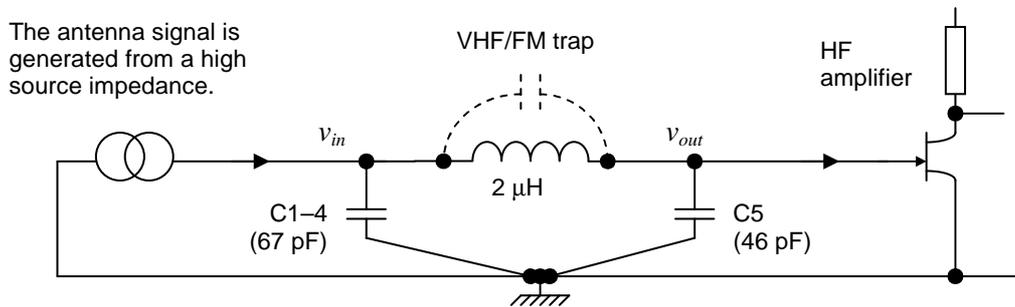
**Figure 6.1:** The VHF/FM Trap and Its Equivalent Circuit
