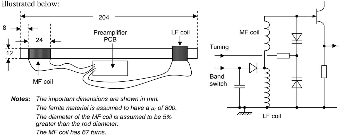
**Figure 7.1:** The LF/MF Antenna Arrangement
