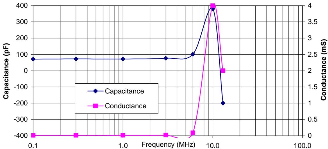
**Figure 4.1:** ‘Strange Effect’ Noted when Measuring Total Input Capacitance
