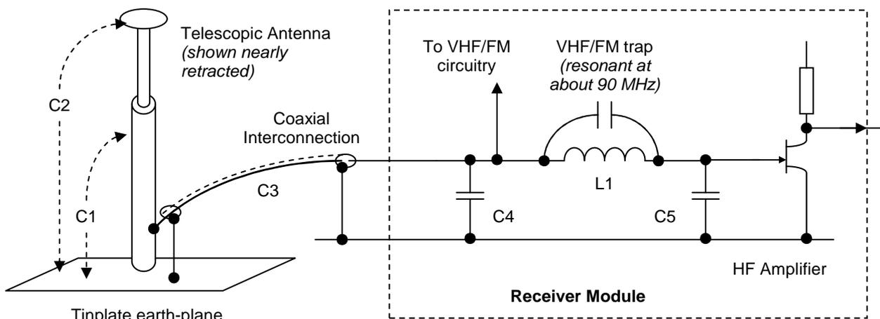
**Figure 3.1:** Telescopic Antenna and Its Associated Circuitry
