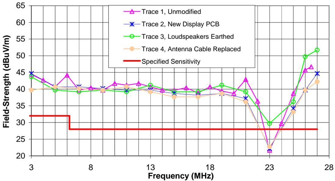
**Figure 5.3:** Typical Sensitivity Measurement Runs
