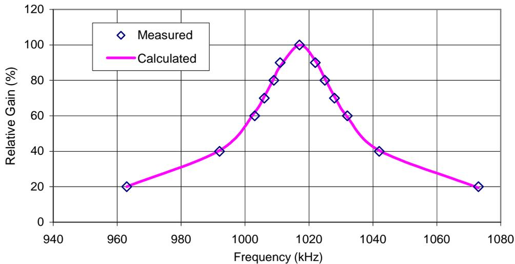
**Figure 8.1:** Response of the MF Antenna, as Found
