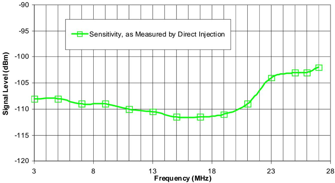
**Figure 5.1: Sensitivity Measured by Means of Direct Injection**
