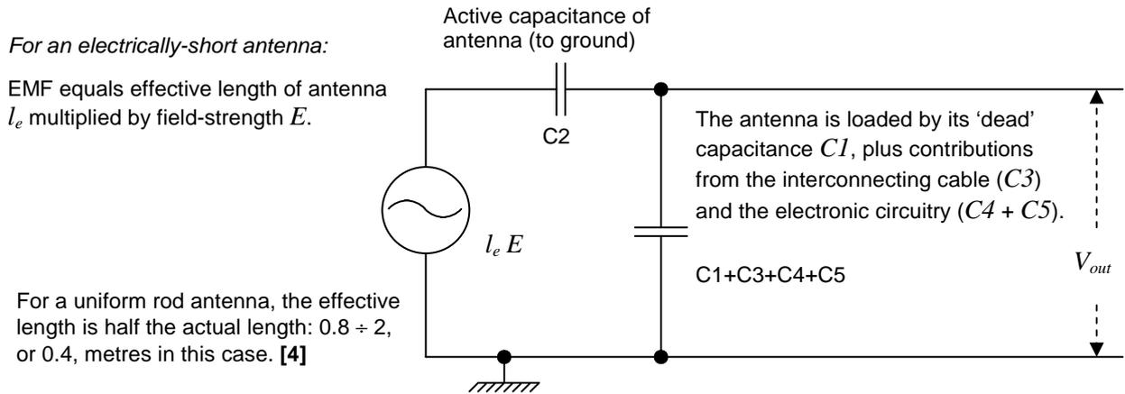
**Figure 5.2: Model for Calculating the Antenna Sensitivity**
