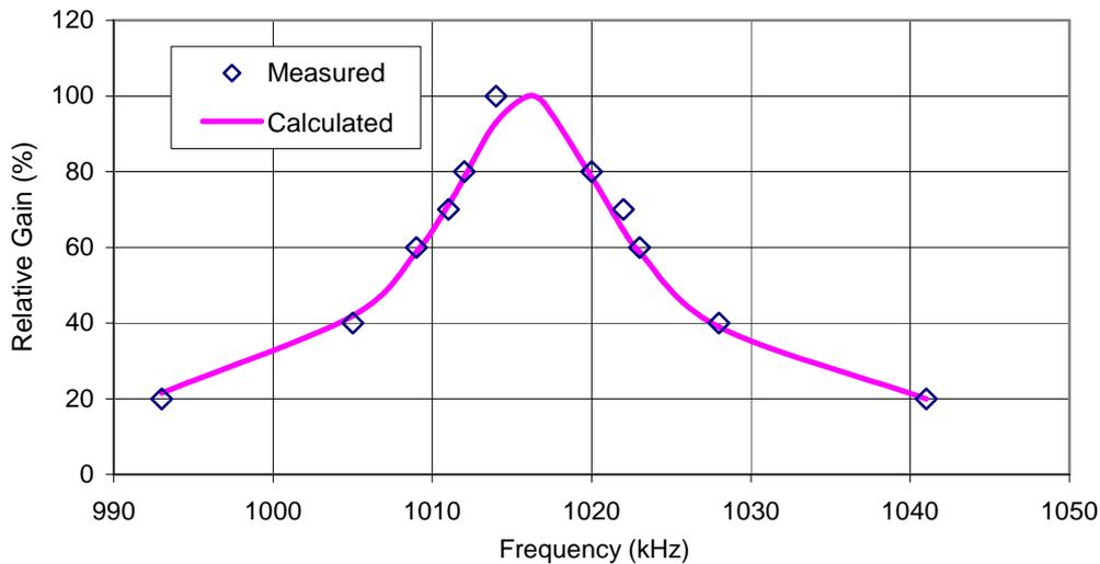
**Figure 9.1:** Response of the MF Antenna, with LF Coil out of Circuit
