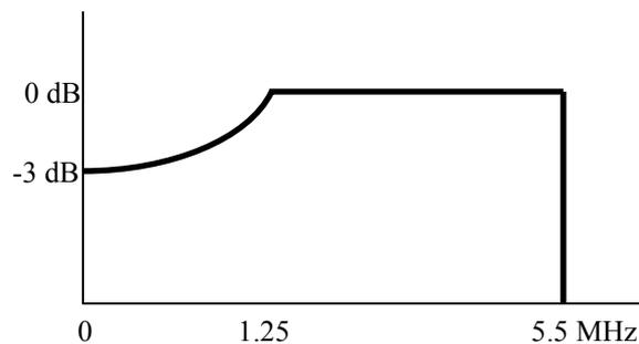
**Figure B1: Noise spectral density from an ideal PAL-I demodulator**
