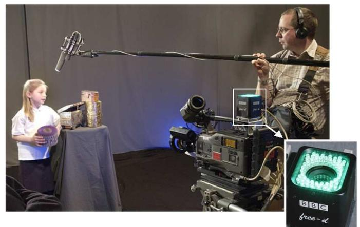
Figure 3. *free-d* tracking camera mounted on studio TV camera.
