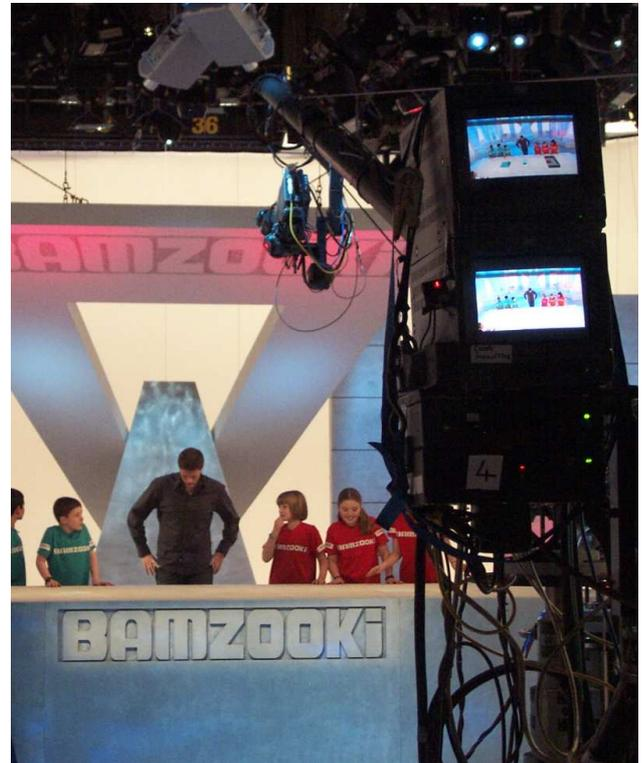
Figure 6. Projection feedback in use on the BBC show *BAMZOOKi* (the monitors on the right show the composite image and the original camera image)
