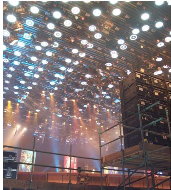
Figure 2. Circular barcoded markers mounted on the ceiling of a TV studio
