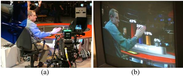
Figure 5. Use of the “FlashKey” technique: (a) shows studio set-up, with strobe light on left, illuminating the presenter’s arm, and (b) shows the composite image after processing.
