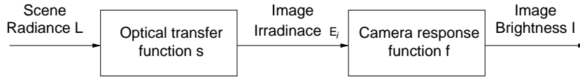
Fig. 1. Flow diagram of the transfer functions s and f that transform the scene radiance into image brightness (adapted from [10]).
