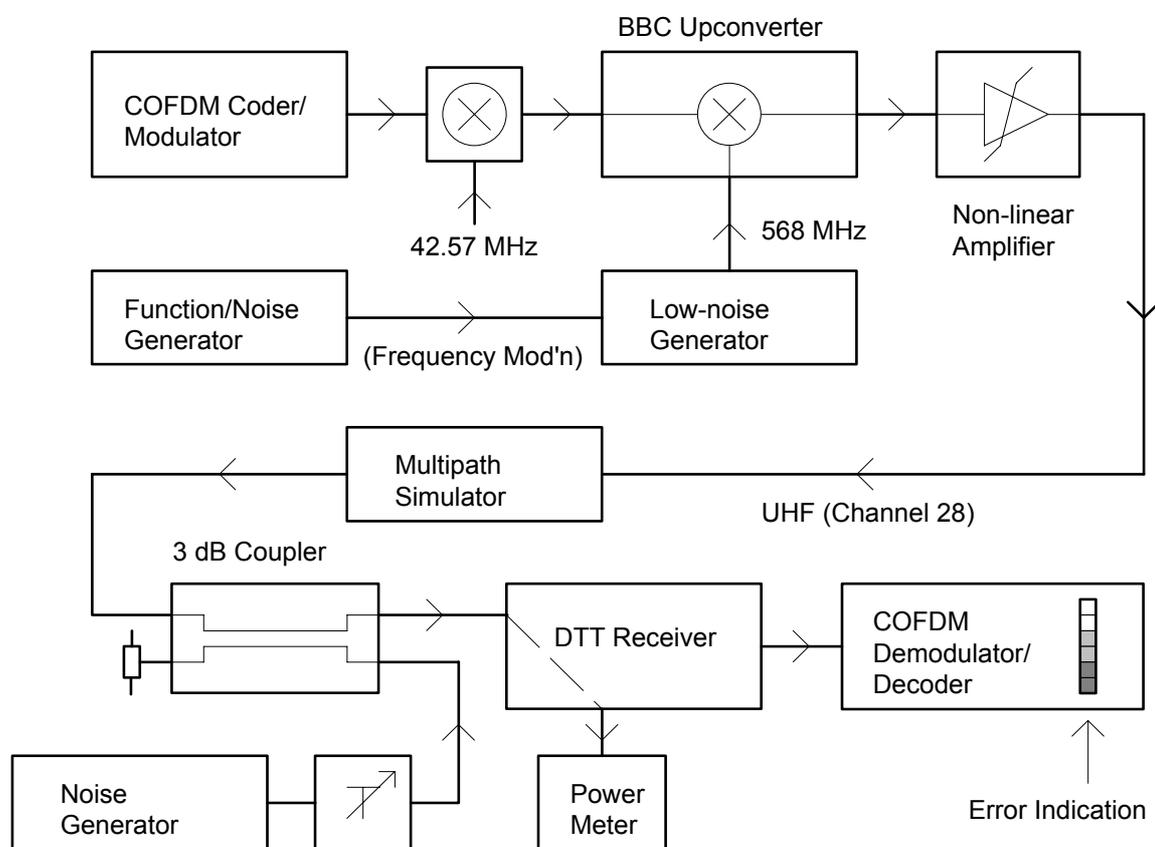
**Figure 3:** Experimental Arrangement for Checking END Theory
