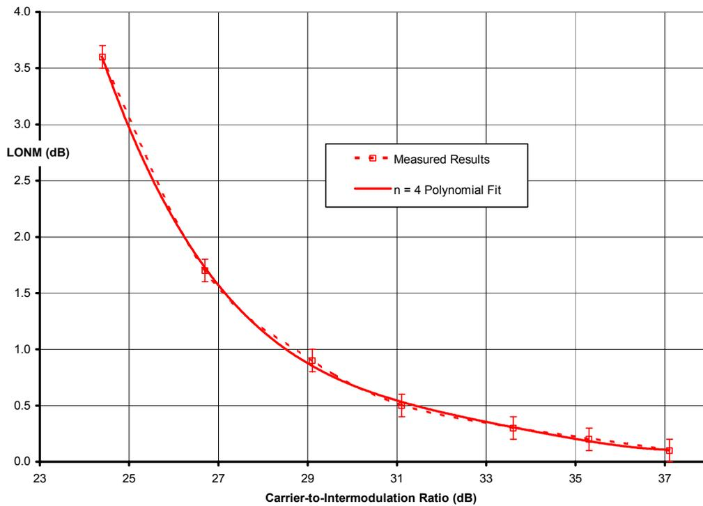
**Figure 5:** END (LONM) versus Carrier-to-Intermodulation Product Level
