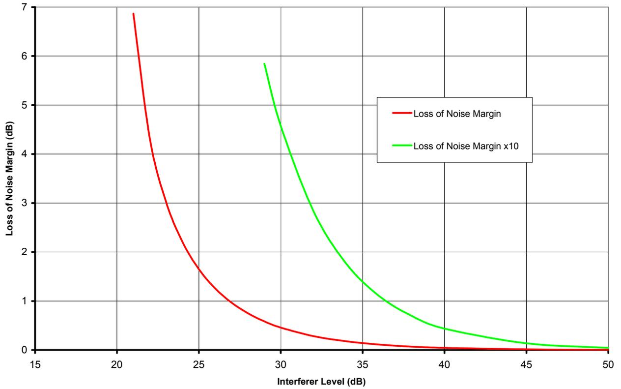
**Chart 1:** Loss of Noise Margin (END) versus Noise-like Interferer Level (ENF)
