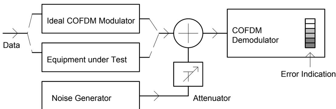
**Figure 1:** Measurement of Equivalent Noise Degradation
