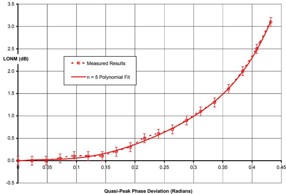
**Figure 4:** END (LONM) versus Local Oscillator Phase Noise Deviation
