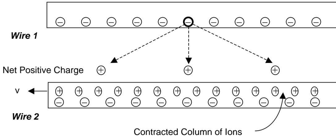
**Figure A1.1:** Illustration of Attraction between Wires Carrying Electric Current
