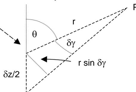
**Figure 2.3:** Current Spreading out from a Doublet
