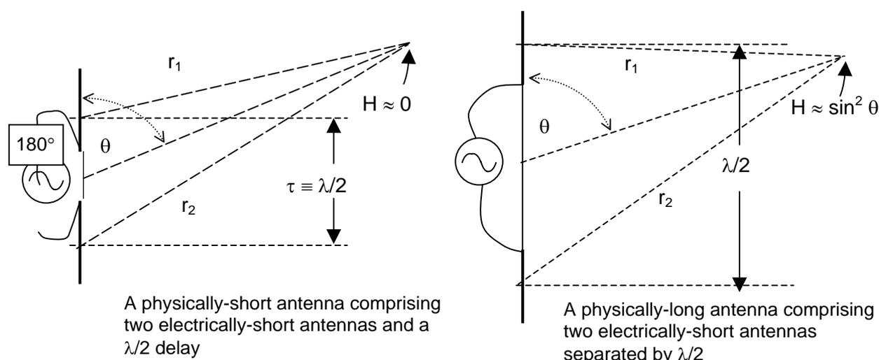
**Figure 5.1:** Comparison of Antennas with Lumped and Distributed Delays
