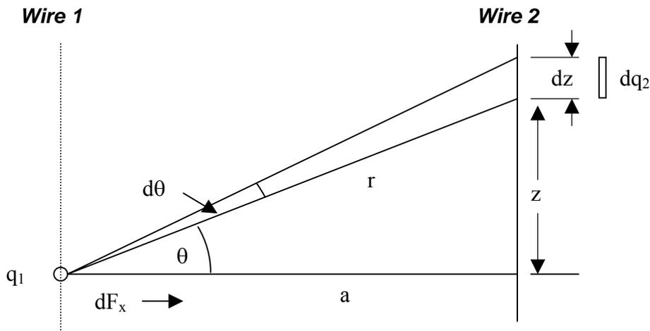
**Figure A1.2:** Calculation of Attraction between Point and Line Charges
