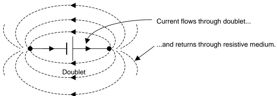
**Figure 2.1:** Current Flow through Doublet and Surrounding Resistive Medium
