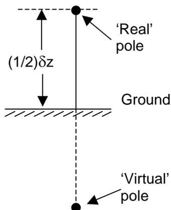
Figure 4.1 illustrates the effect of the ground. At actual transmitting stations, the ground conductivity is enhanced in the neighbourhood of the antenna, usually by burying radial copper strips to form an ‘earth-mat’. The transmitter power is then applied between the earth-mat and the antenna.
