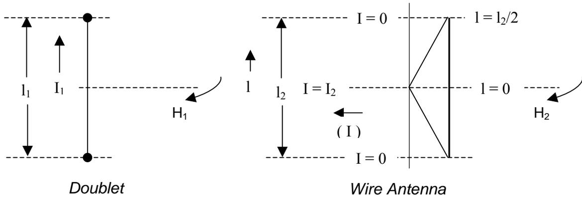
**Figure 4.2:** Comparison of Doublet and Wire Antennas
