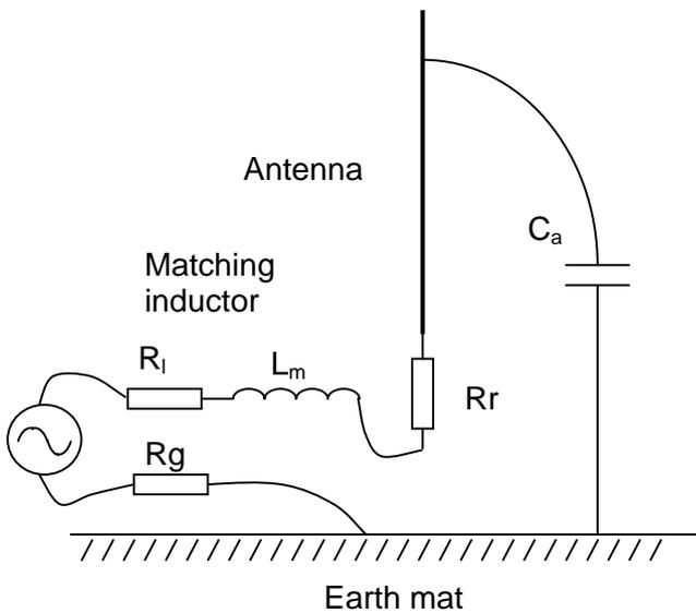
Figure 5.2 shows the antenna, which possesses a radiation resistance of  $R_r$  ohms and capacitance  $C_a$ . The effective ground resistance is  $R_g$ . Since the transmitter will probably wish to ‘see’ a resistive load,  $C_a$  is shown neutralised by inductor  $L_m$ . The equivalent series resistance of the inductor is  $R_1$ .
