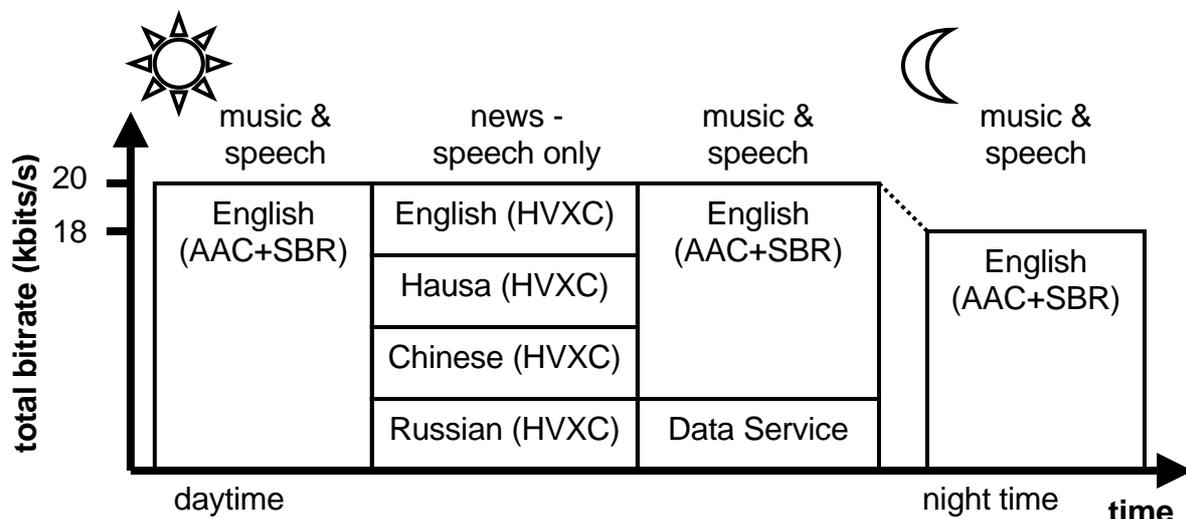
Figure 1 – Possible configurations of a MW DRM transmission
