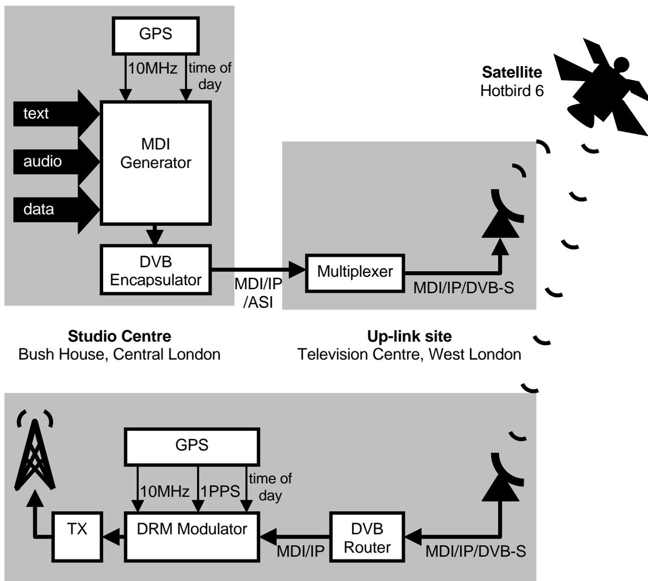
Figure 3 – The DRM distribution network in use by the BBC World Service
