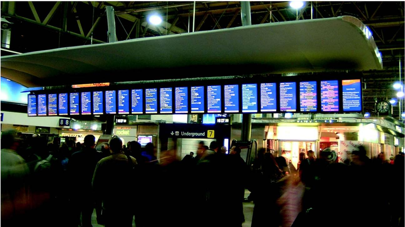
PDPs used as data displays in a major UK railway station. This photo indicates the brightness/contrast problem, which has had to be cured by placing ever larger canopies above the displays to block light coming in from the glass roof above, during daylight hours.
