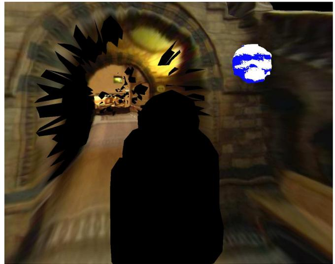
Fig. 14. Projected image. The black region in the bottom-centre is the mask generated from the 3D surface model.
