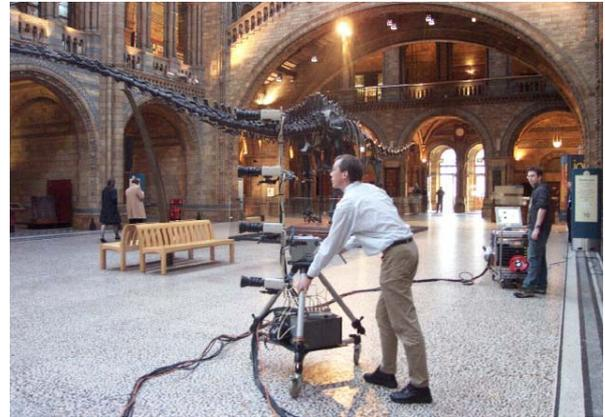
Figure 3 – image data acquisition with multi camera rig
