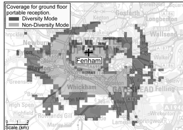
Figure 12: The improvement to indoor coverage by the use of antenna diversity
