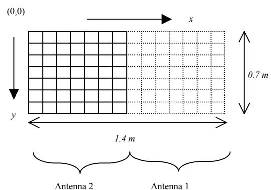
Figure 7: A matrix of measurements using two antennas
