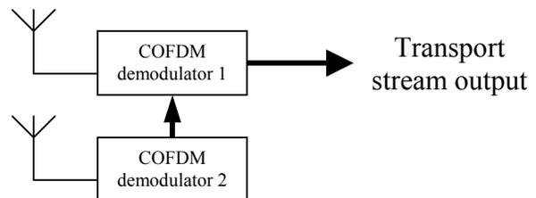
Figure 1: Connection of two demodulators for diversity
