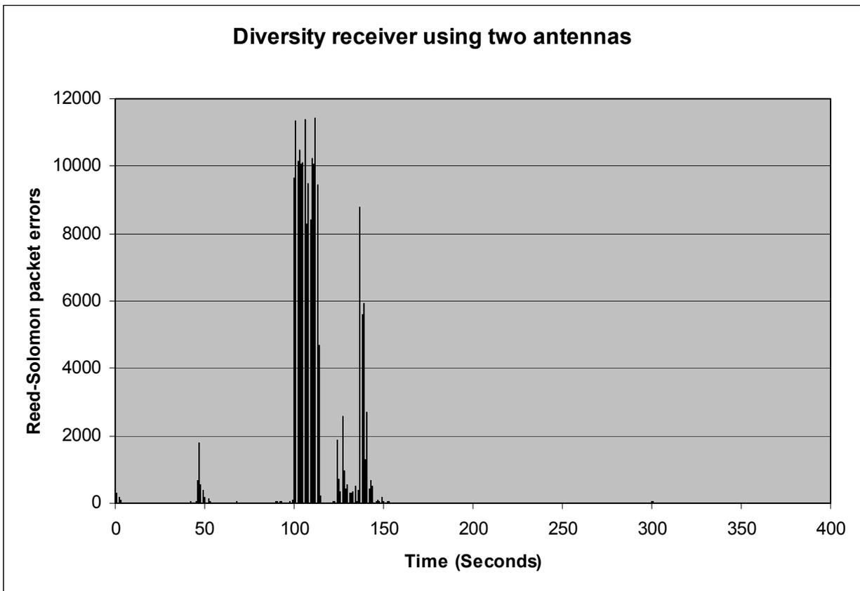
Figure 5: Number of packet errors per second using a diversity receiver with two antennas
