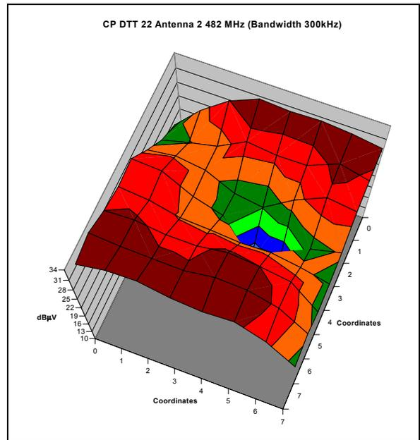
Figure 9: Signal level measured on antenna 2 in a bandwidth of 300 kHz
