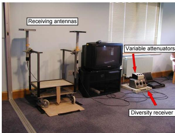
Figure 11: A typical measurement set-up.
