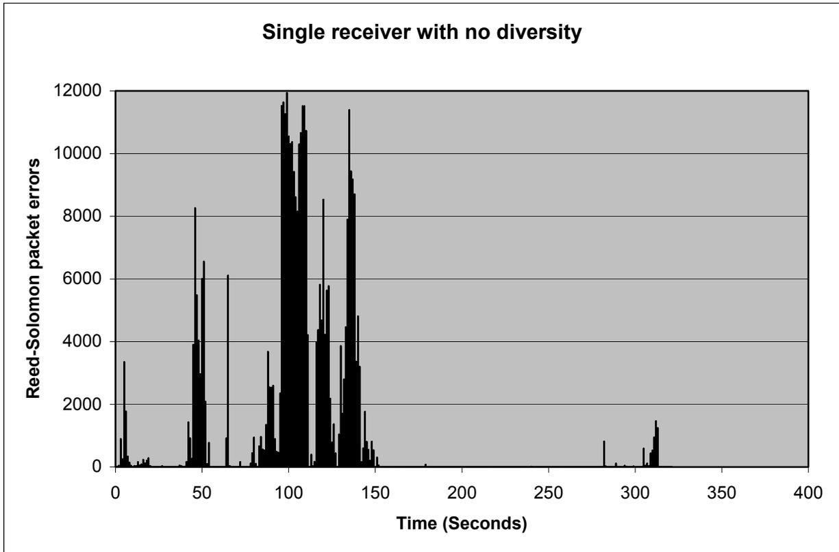
Figure 4: Number of packet errors per second without using diversity
