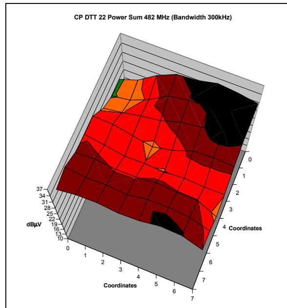
Figure 10: Power sum of the signal levels measured on the two antennas
