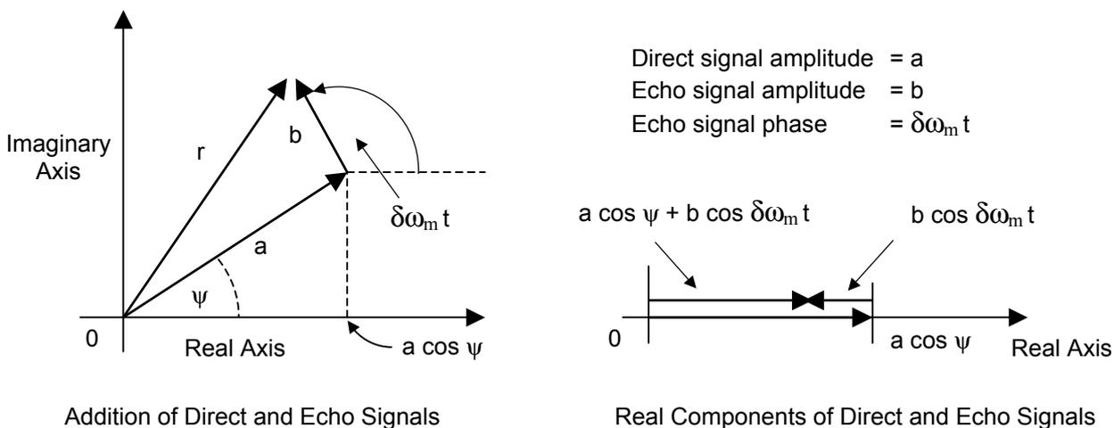
**Figure 2.2** Addition of Direct and Echo Signal Vectors
