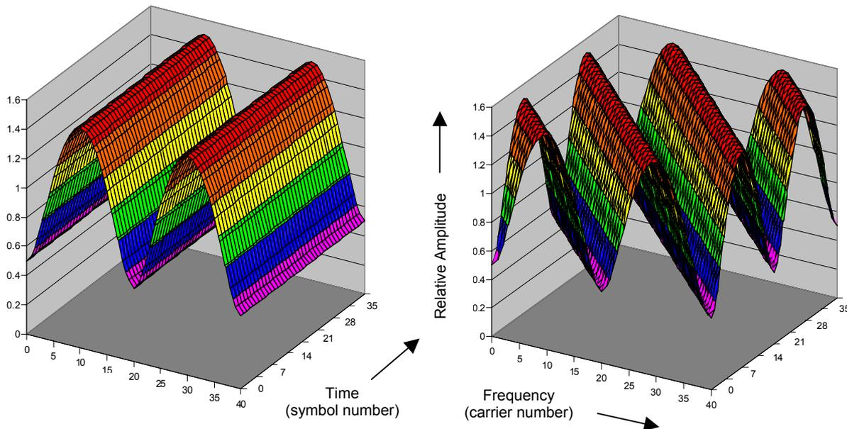
**Figure 2.1:** Illustration of the Effect of Doppler on the Channel Response
