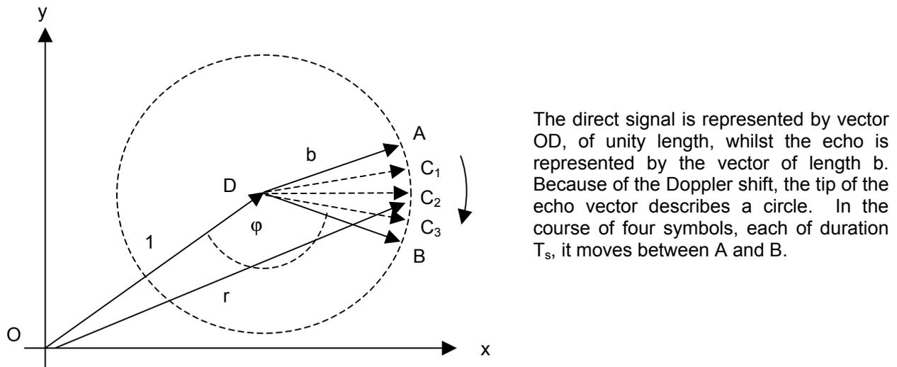
**Figure 3.1:** Illustration of the Time Variation of a Single Carrier
