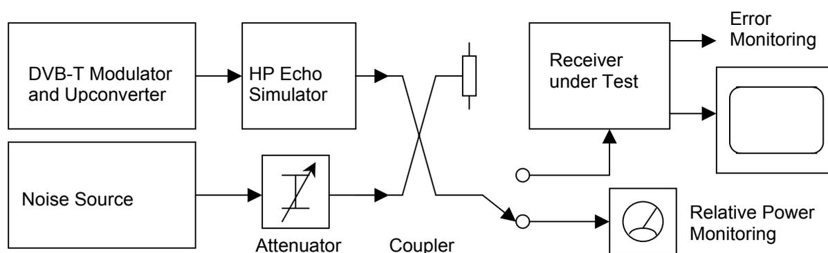
**Figure 5.1:** Experimental Arrangements for Measuring Equivalent Noise Degradation
