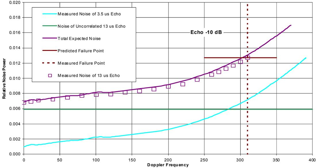
**Figure 8.1:** Noise Associated with a Doppler-shifted, 13.05  $\mu\text{s}$  Delay Echo
