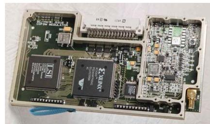
Fig 2. DVB-T modulator and I/Q upconverter card
