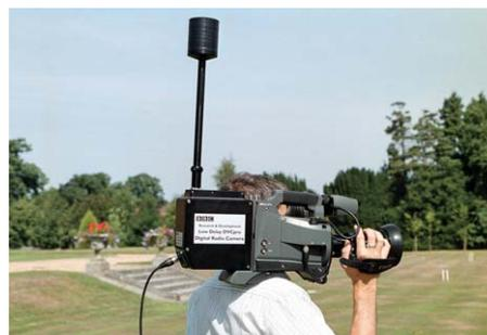
Fig. 1. BBC Digital Radio Camera
