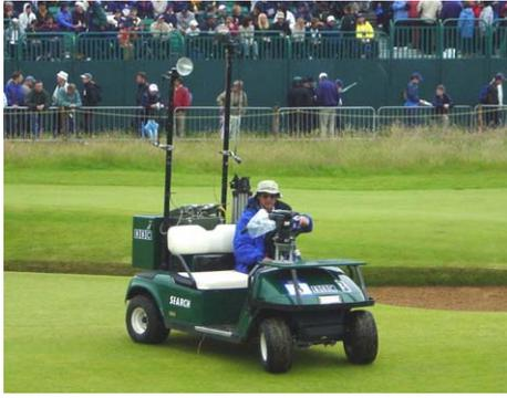
Fig 3. A golf buggy used as a moveable relay
