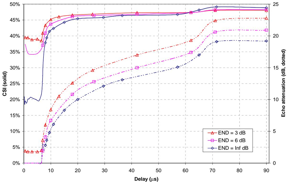
Figure 4: Average CSI and echo attenuation corresponding to  $BER_{REF}$  for a 2-path channel plotted as a function of the echo delay and the Equivalent Noise Degradation (END).
