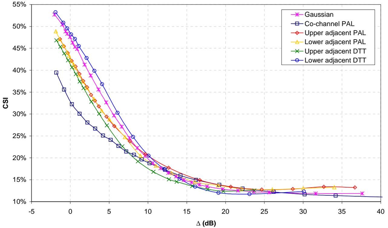
Figure 3: Average CSI for the six types of interference shown in the inset box. The variable  $\Delta$  is the variation in C/I with respect to  $C/I_{\text{REF}}$  for each impairment.
