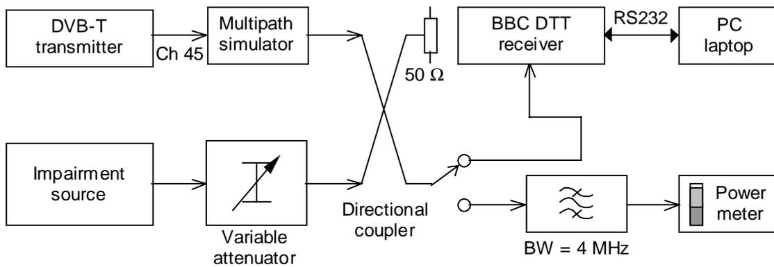
Figure 1: Lab set-up used to measure DVB-T performance.
