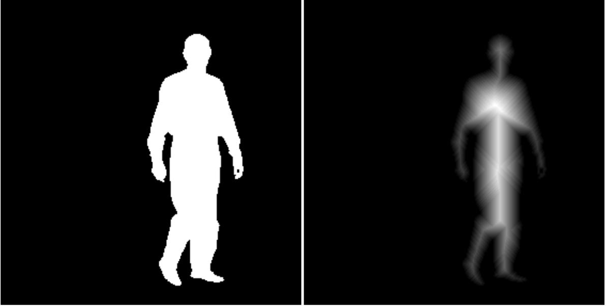
**Figure 4.** Silhouette mask created by chroma-keying (left), metric of boundary distance (right)
