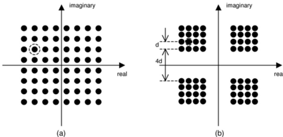
**Figure 1 Constellations of 64-QAM DVB-T signals**
