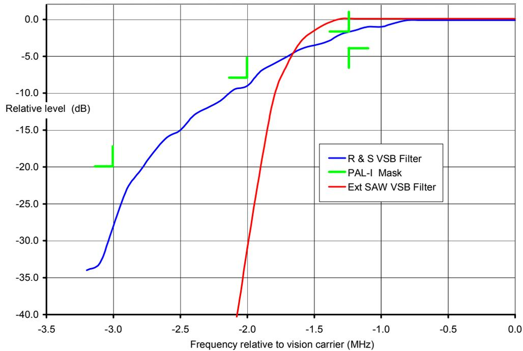
**Figure 6:** Sideband Response of the Modulator with the Two Alternative VSB Filters<sup>7</sup>
