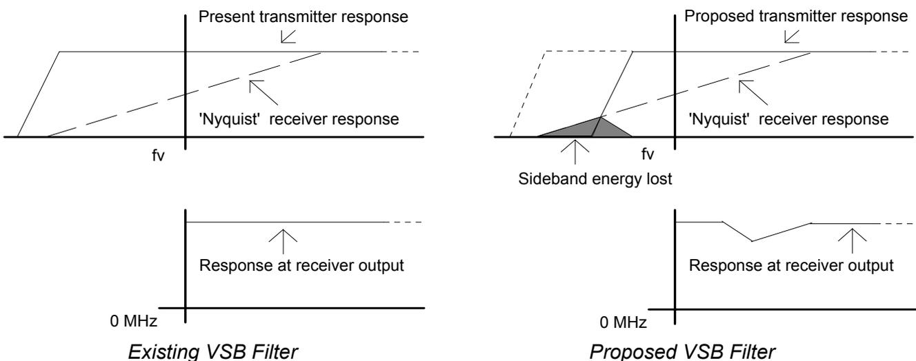
**Figure 2:** The Effect of Reducing the Transmitted Vestige
