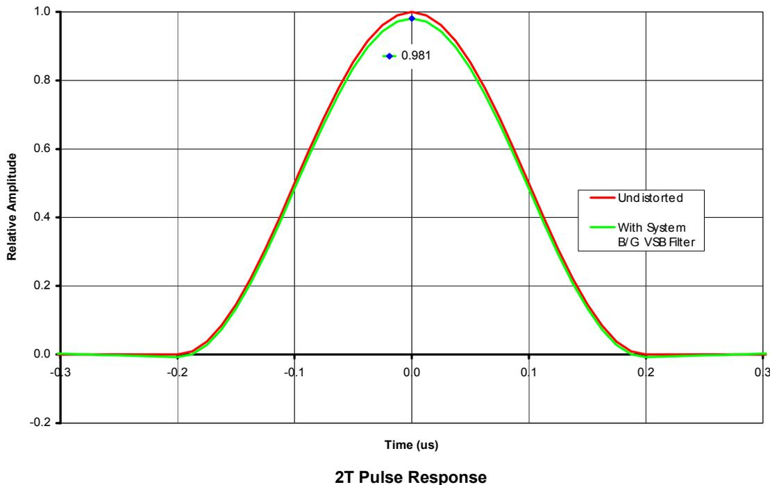
**Figure 4:** The Distorted 2T Pulse Resulting from Reduction of the Transmitted Vestige
