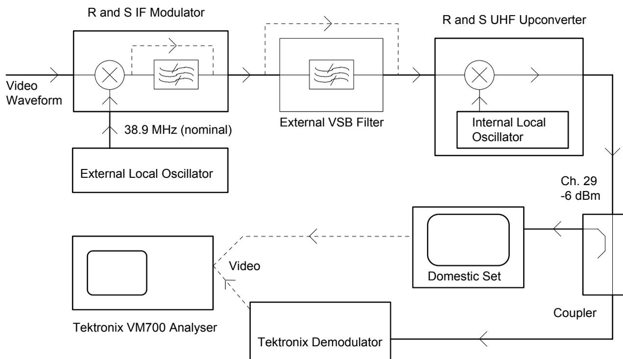
**Figure 5:** Arrangements for Assessing the Effects of PAL-I Vestige Reduction
