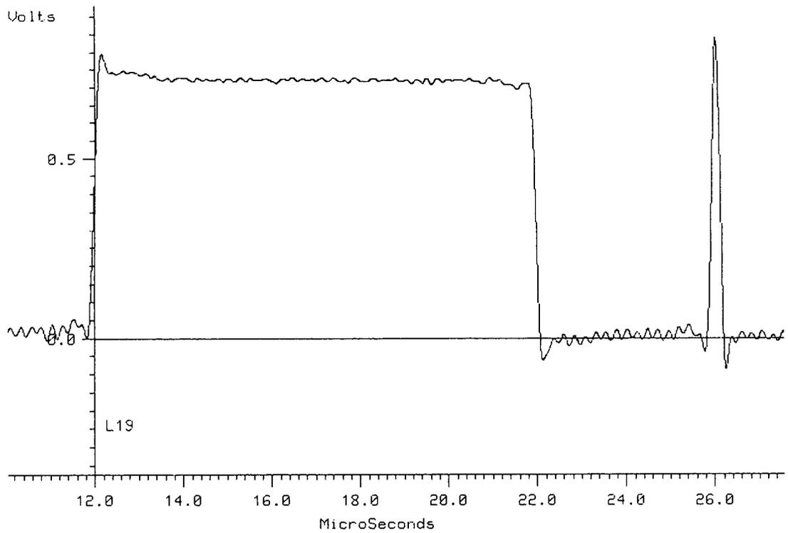
**Print 6: 2T Pulse and Bar at Output of Domestic Receiver
