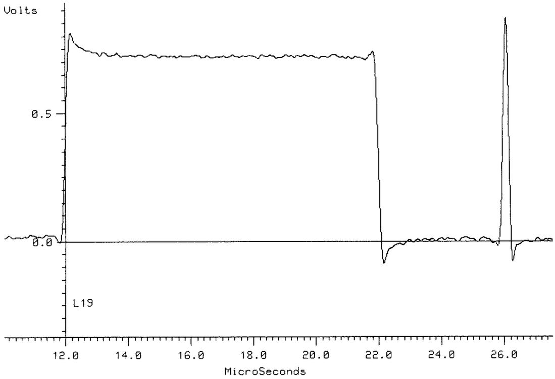
**Print 5: 2T Pulse and Bar at Output of Domestic Receiver
