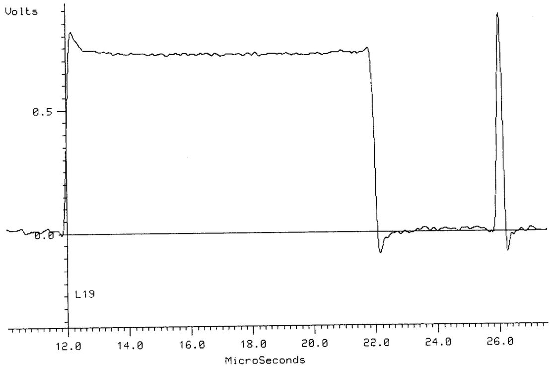
**Print 4: 2T Pulse and Bar at Output of Domestic Receiver
