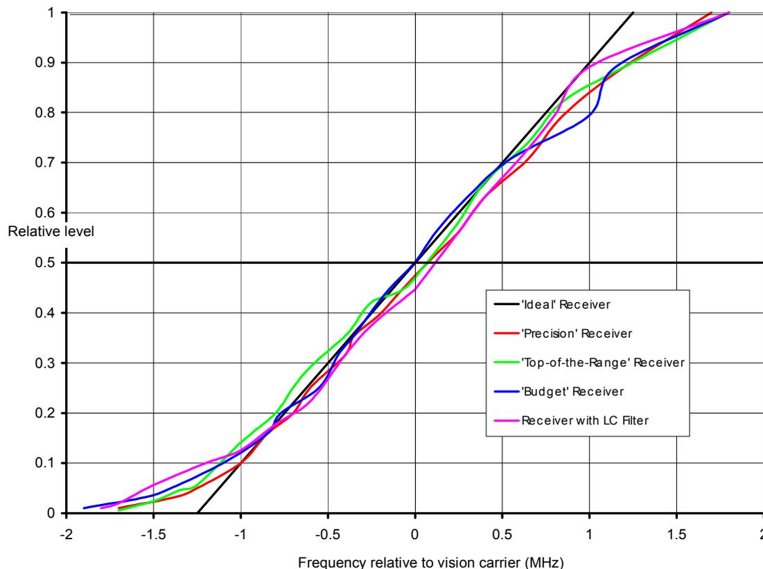
**Figure 8:** Nyquist Filter Responses of the Receivers Tested
