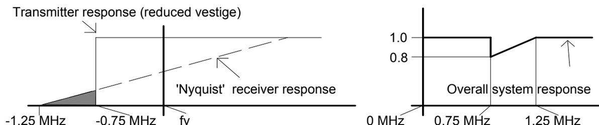
**Figure 3:** The System Response Resulting from a Simulated Reduction of Transmitted Vestige
