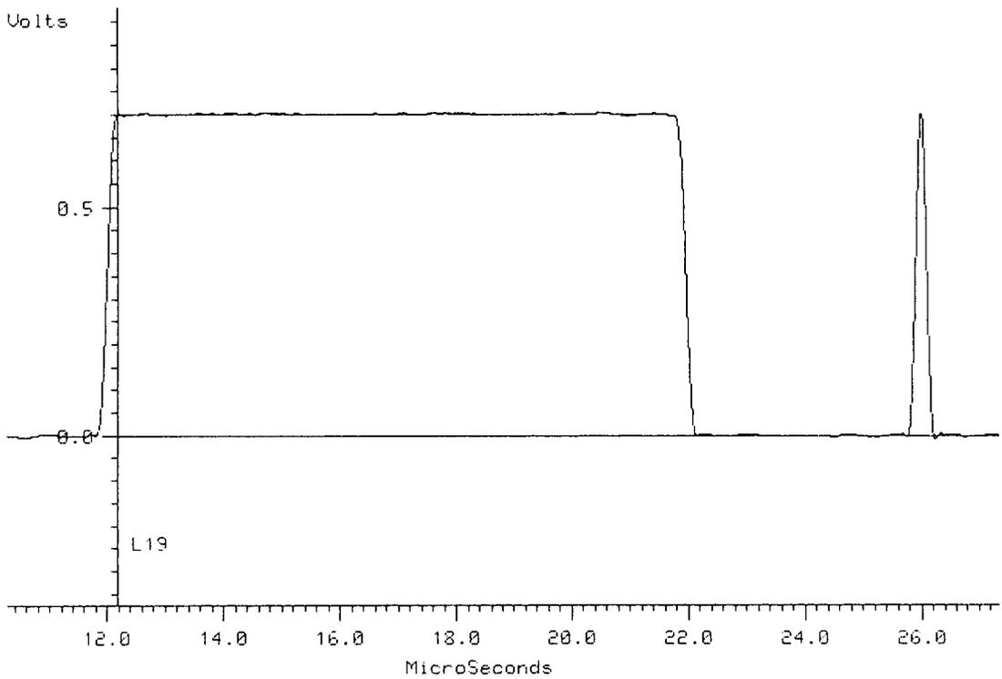
**Print 2: 2T Pulse and Bar at Output of Precision Receiver**
