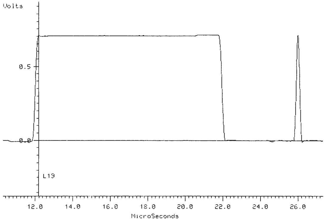
**Print 1: 2T Pulse and Bar at Output of Precision Receiver**
