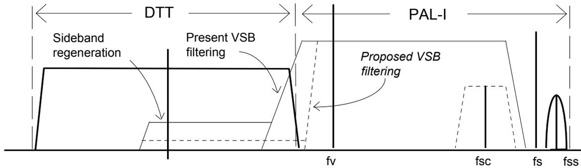
**Figure 1:** Typical Adjacent Channel PAL-I and DTT Spectra
