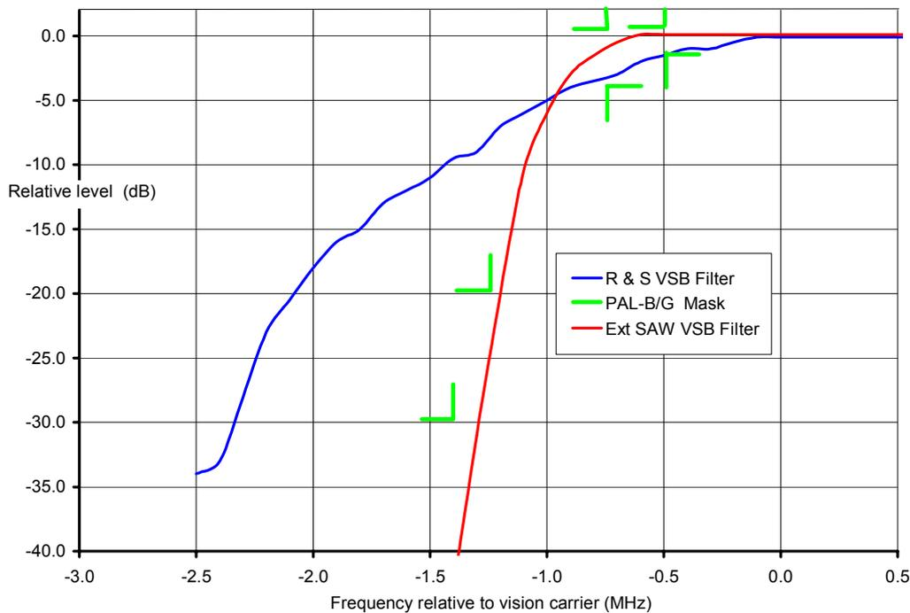
**Figure 7:** Sideband Response of the Modulator when Optimised for System B/G
