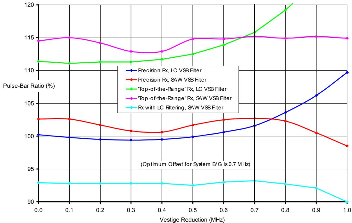
**Figure 9:** 2T Pulse-to-Bar Ratio as a Function of Vestige Reduction
