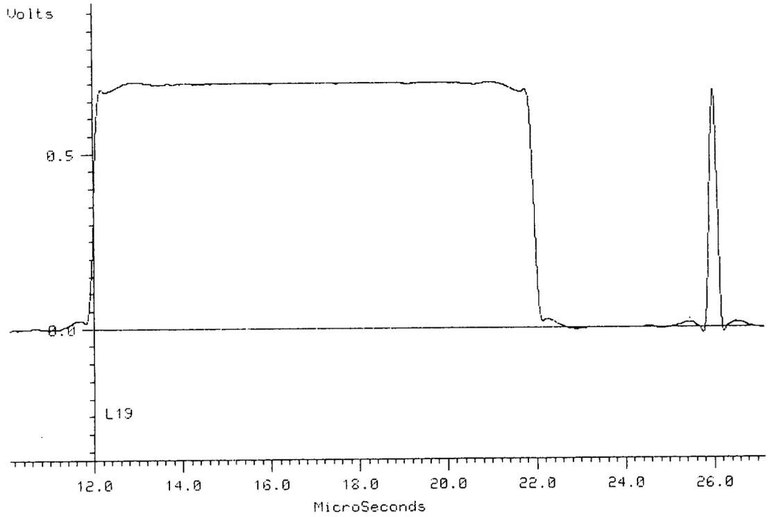
**Print 3: 2T Pulse and Bar at Output of Precision Receiver
