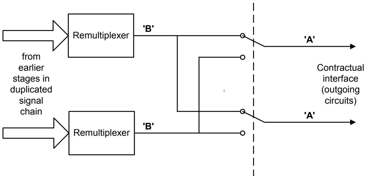
Figure 1 - Connection of the Bitmon probes at the studio-centre outputs
