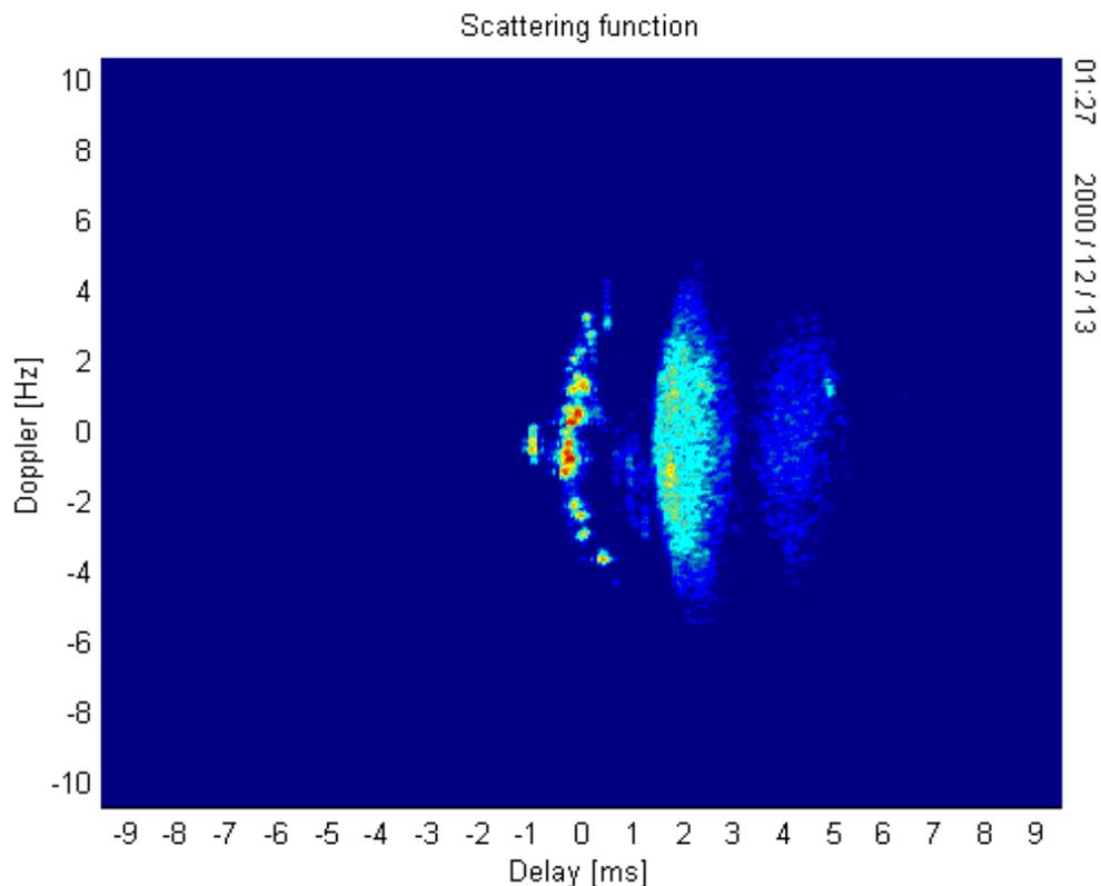
Figure 1 – NVIS scattering function. The colours depict a range of 40 dB.
