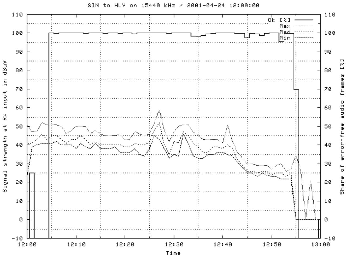
Figure 4 - Example of graph showing the evolution of signal strength and audio quality. Transmission from Sines (Portugal) to Hilversum (NL).
