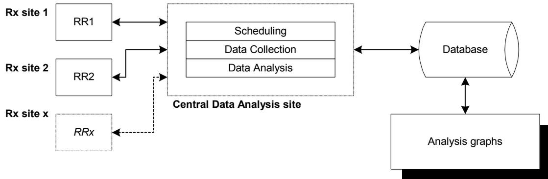
Figure 3 - Data flow between remote receivers and central data analysis site
