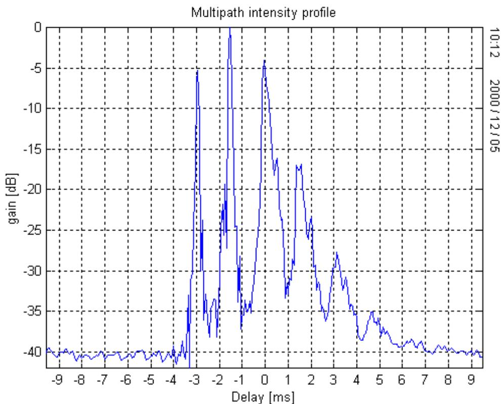
Figure 2 - Delay Spectrum of a benign NVIS reception in Ecuador
