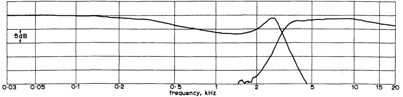
Fig. 2 - Voltages applied to l.f. and h.f. units
