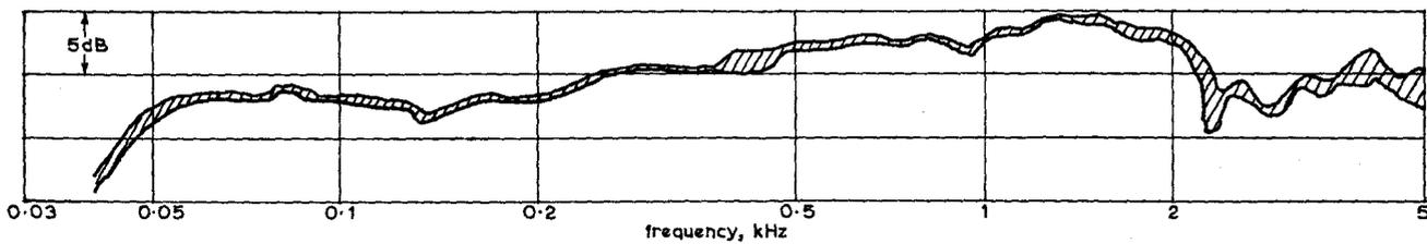
Fig. 7 - Spread in axial response/frequency characteristics of eight unequalized low-frequency units
