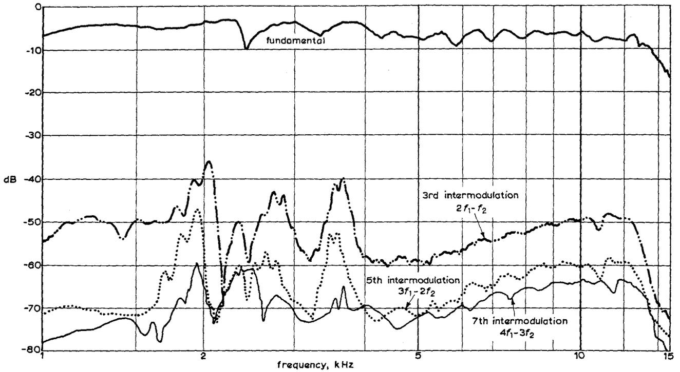
Fig. 5 - Measurements of intermodulation distortion with frequencies  $f_1$  and  $f_2$  and a sound level of  $1 \text{ N/m}^2$  at 1.5 m on axis
