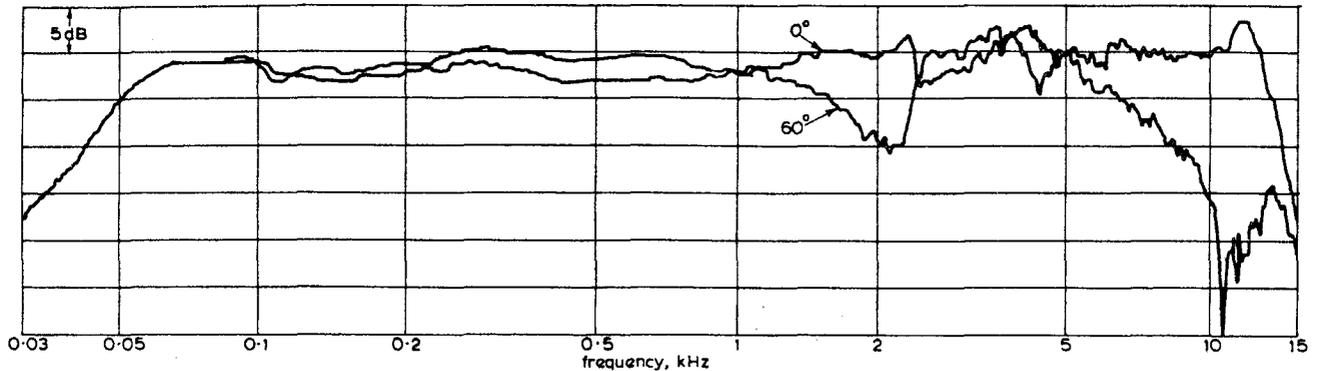
Fig. 3 - Response/frequency characteristics of complete loudspeaker. Curves at  $0^\circ$  and  $+60^\circ$  in vertical plane
