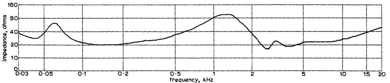
Fig. 6 - Modulus of impedance
