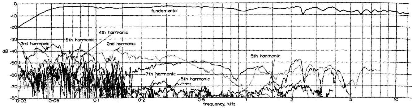
Fig. 4 - Measurements of harmonic distortion for a sound level of  $1 \text{ N/m}^2$  at 1.5 m on axis
