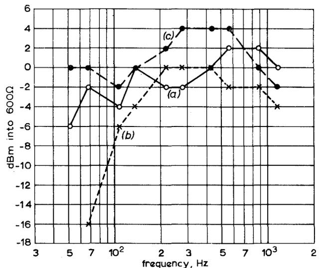
Fig. 2 - Peak levels in octave analysis of programme
