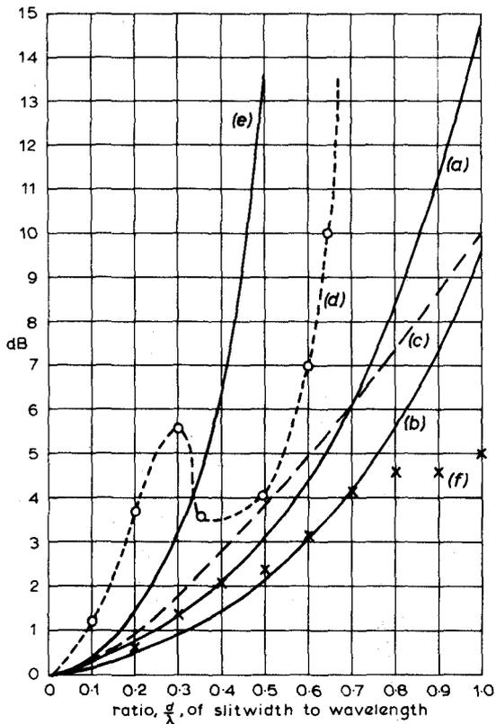
Fig. 6 - Deviation of 60° characteristics from axial characteristics for differing types of source
