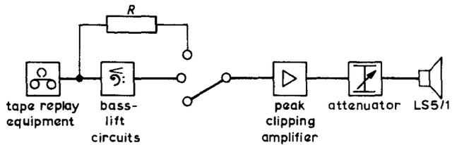
Fig. 4(b) - Circuit used for determination of acceptable distortion with bass-lift circuits
