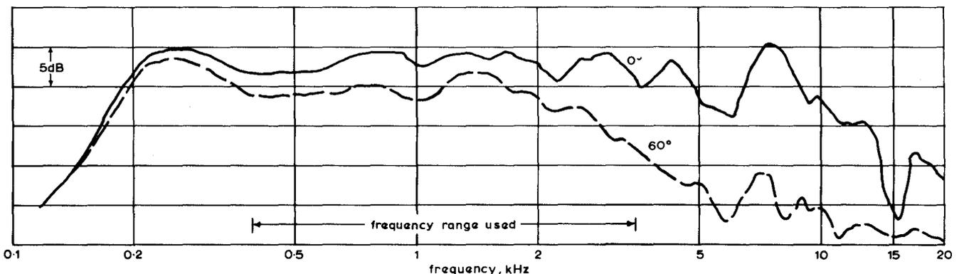
Fig. 8 - Response/frequency characteristic of 200 mm dia. middle-frequency unit without slit at  $0^\circ$  and  $60^\circ$  to the axis
