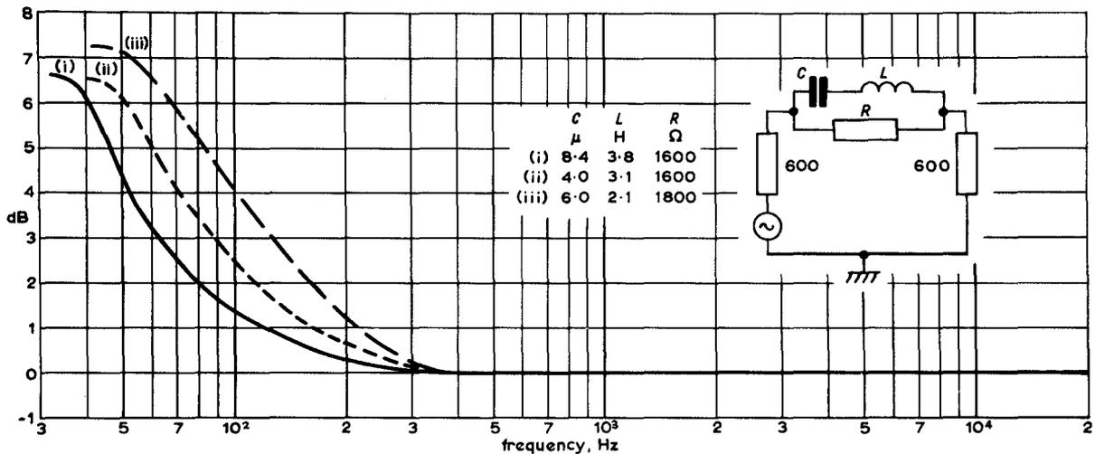
Fig. 4(a) - Response/frequency characteristics of bass-lift circuits
