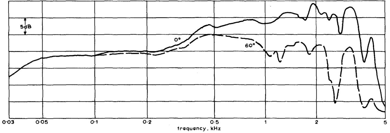
Fig. 5(a) - Response/frequency characteristic of unequalized low-frequency unit without slit at 0° and 60° to the axis
