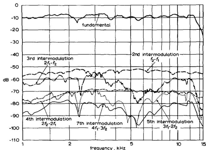
Fig. 23 - Intermodulation distortion of LS5/5 loudspeaker measured at  $1 \text{ N/m}^2$  at 1.5 m
