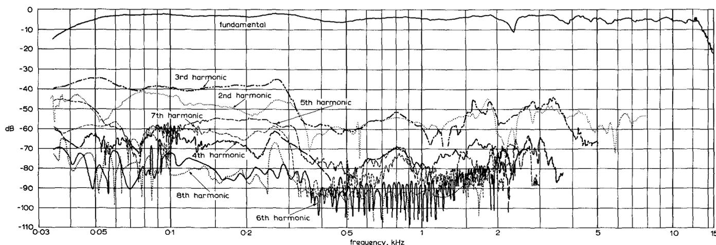
Fig. 22 - Harmonic distortion of LS5/5 loudspeaker measured at  $1 \text{ N/m}^2$  at 1.5 m
