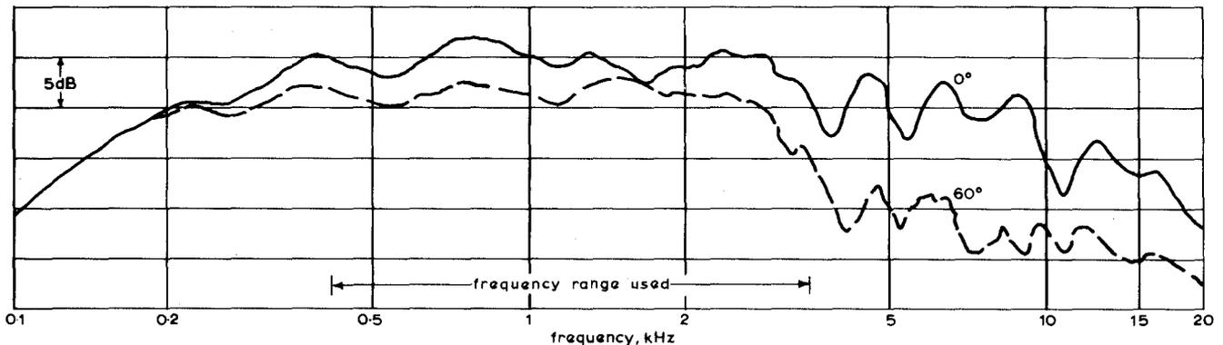
Fig. 7 - Response/frequency characteristics of 110 mm dia. middle-frequency unit at  $0^\circ$  and  $60^\circ$  to the axis
