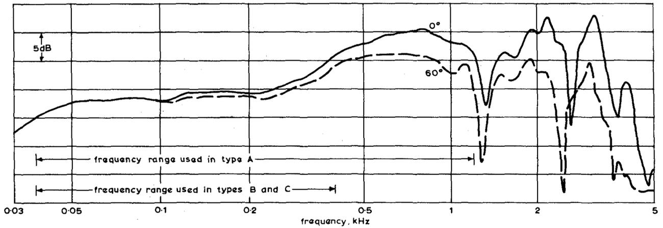
Fig. 5(b) - Response/frequency characteristic of unequalized low-frequency unit with 100 mm slit at 0° and 60° to the axis
