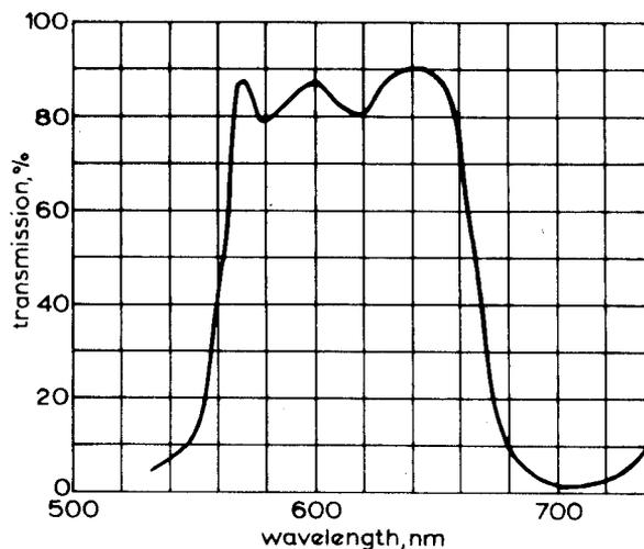
Fig. 2 Interference filter to amend red channel response of telecine.
