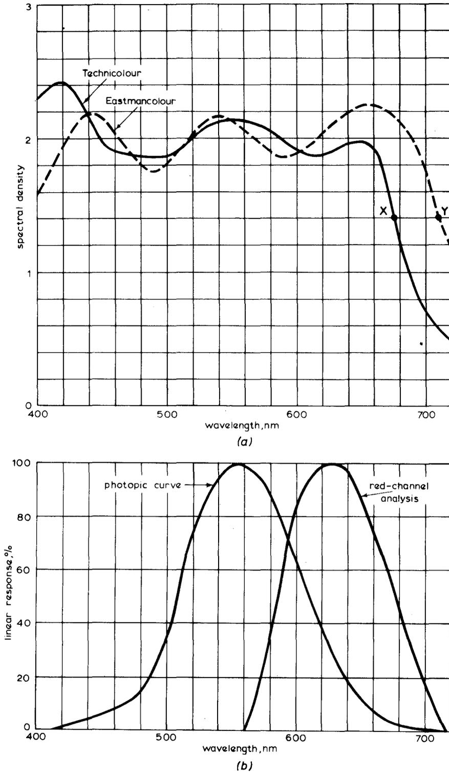
Fig. 1- Comparison of Spectral densities of film stocks with eye response and telecine red-channel response.
