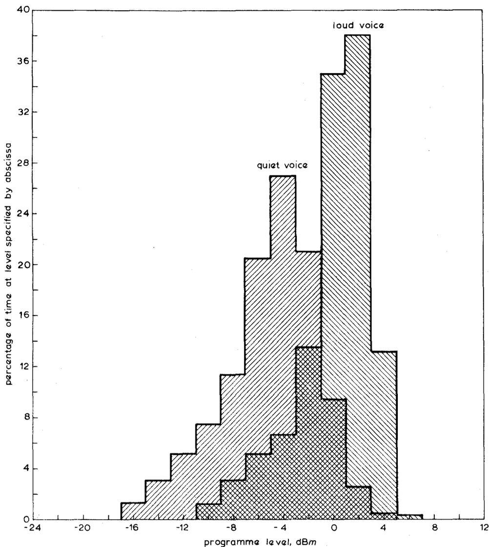
Fig. 10 - Level distribution of voices after passage through 2 : 1 compressor, with 12 dB maximum gain reduction
