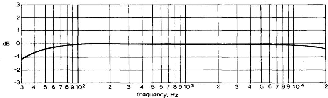
Fig. 5 - "Audimax II RZ" amplifier : frequency characteristic of control chain
