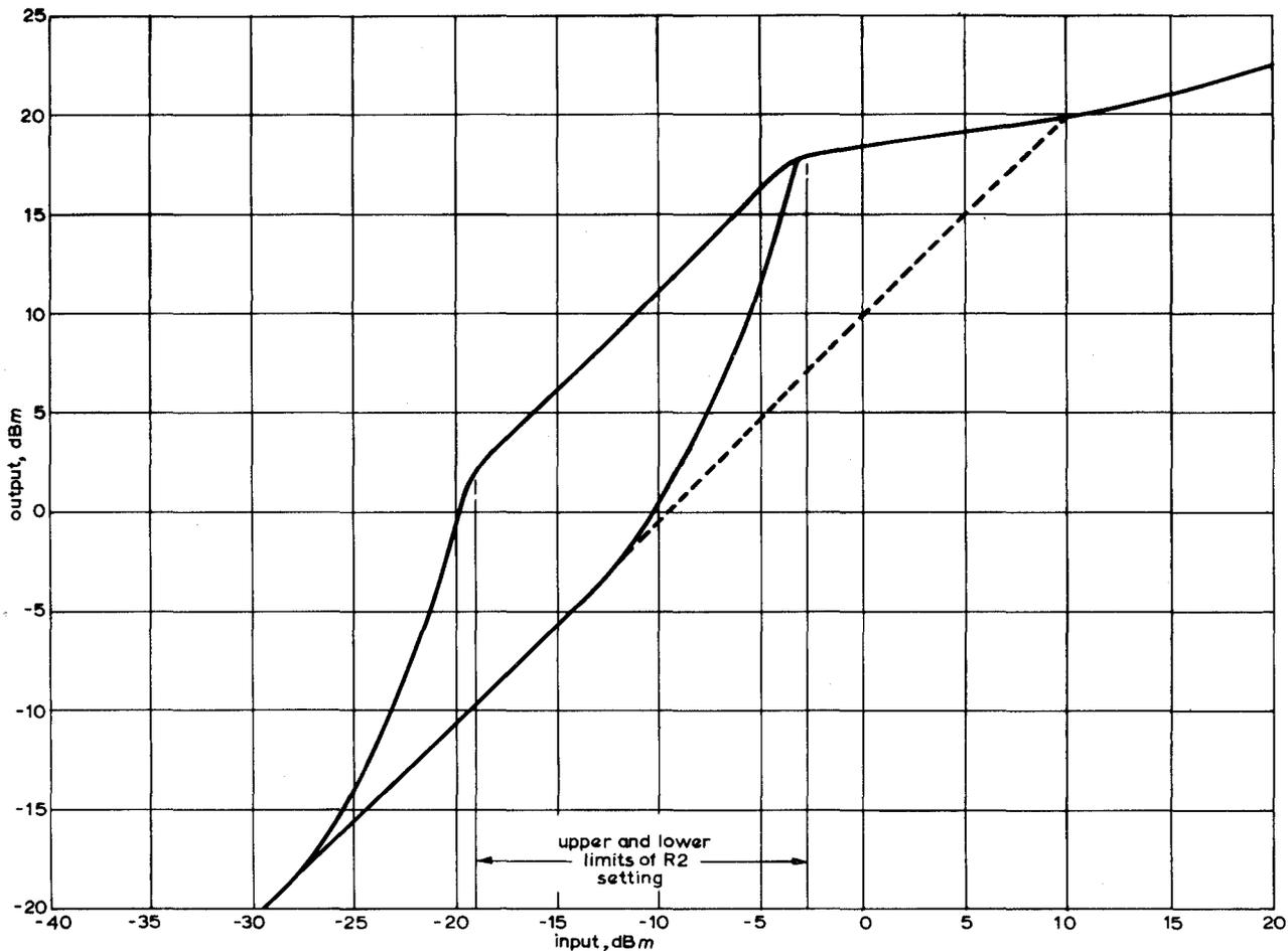
Fig. 3 - "Audimax II RZ" amplifier : output/input characteristic under steady-state conditions
