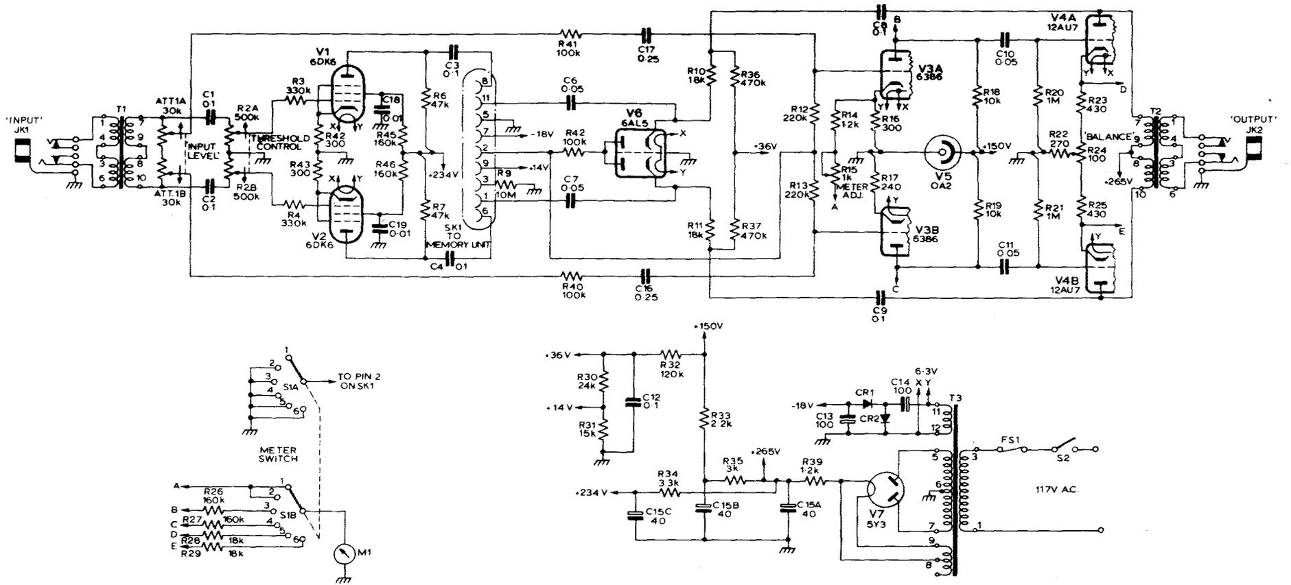
Fig. 1 - "Audimax II RZ" amplifier : circuit diagram
