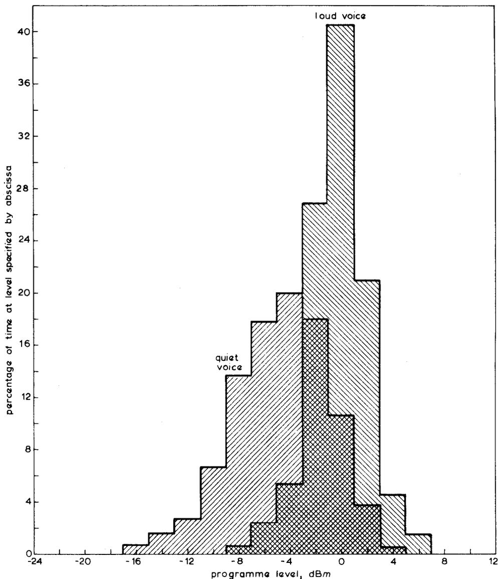
Fig. 9 - Level distribution of voices after passage through LIM/6 with 12 dB maximum gain reduction
