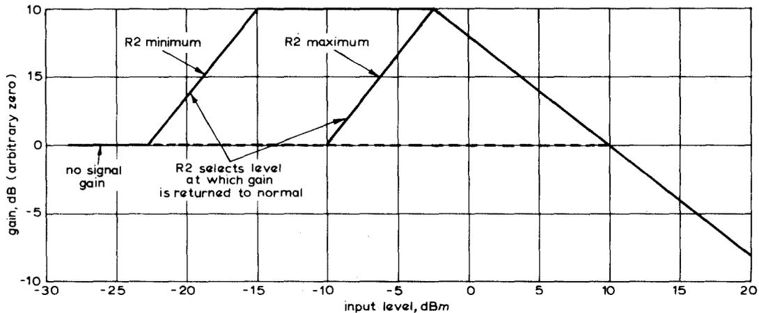
Fig. 2 - "Audimax II RZ" amplifier : variation of gain with input level under steady-state conditions (diagrammatic form)
