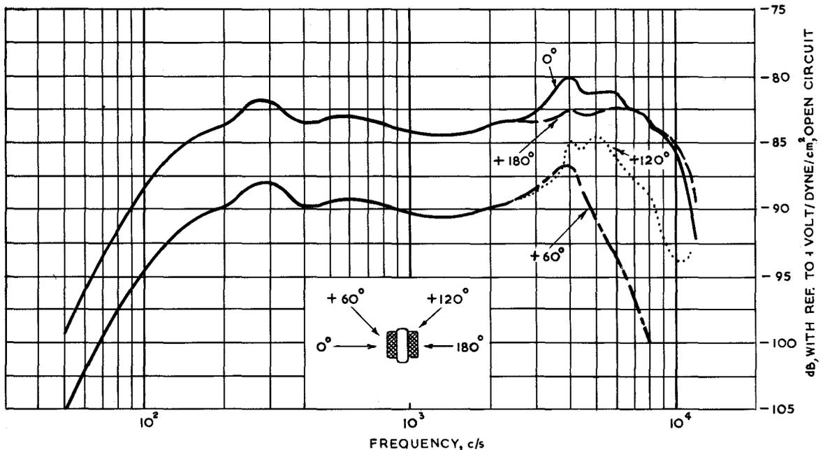
Fig. 4 - Microphone type VRM/T (Specimen A). Frequency characteristics for sound incident at various angles in the horizontal plane
