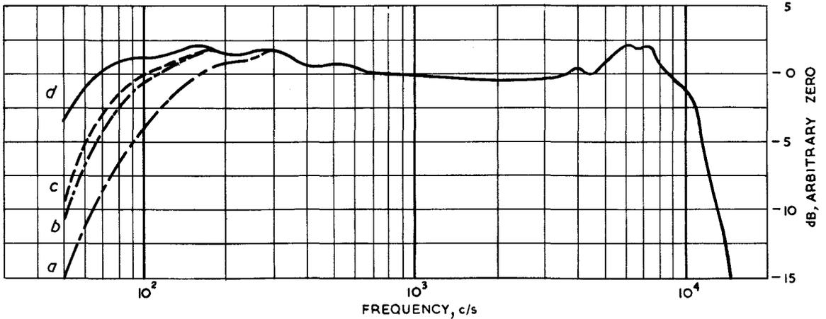
**Fig. 5 - Microphone type RBM/T modified (Specimen B). Axial response curves showing effects of modifications affecting low frequency performance**
