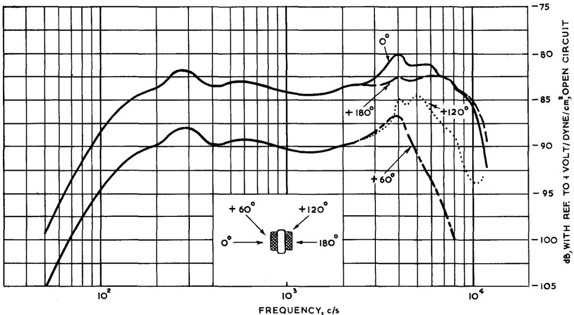
Fig. 4 - Microphone type RBM/T (Specimen A). Frequency characteristics for sound incident at various angles in the horizontal plane
