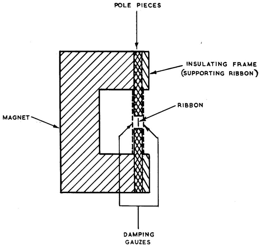
Fig. 3 - Microphone type RBM/T. Section through magnet assembly
