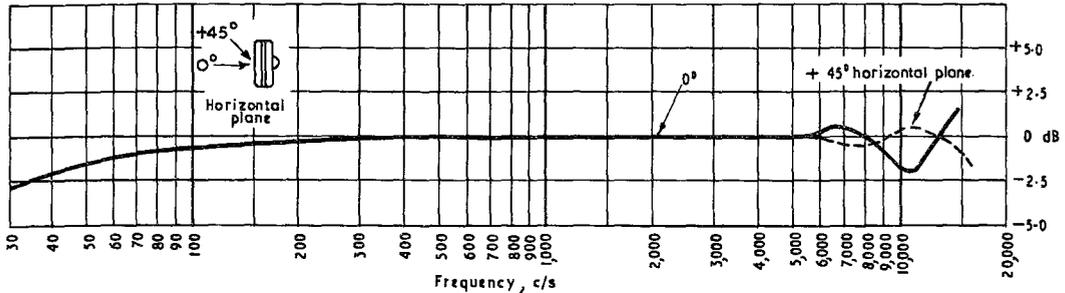
Fig. 4 - Microphone Type PGS. Change in response produced by case
