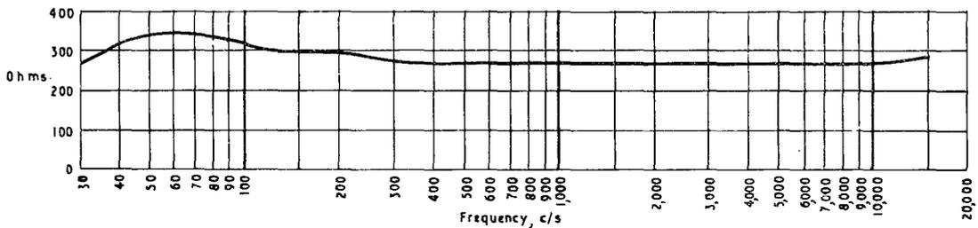
Fig. 10 - Microphone Type PGS. Modulus of output impedance
