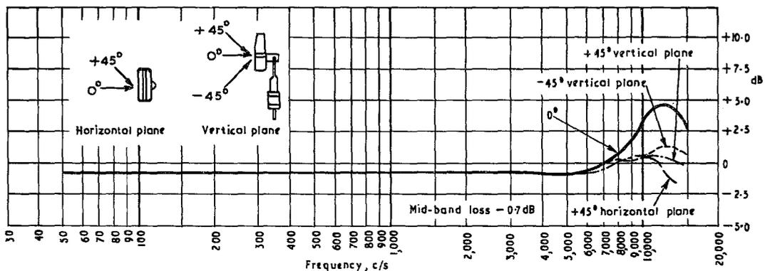
Fig. 5 - Microphone Type PGS. Change in response produced by high-frequency reflectors
