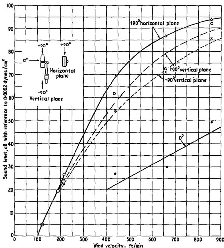
Fig. 11 - Microphone PGS. Weighted wind noise output expressed as equivalent sound level at 1 kc/s
