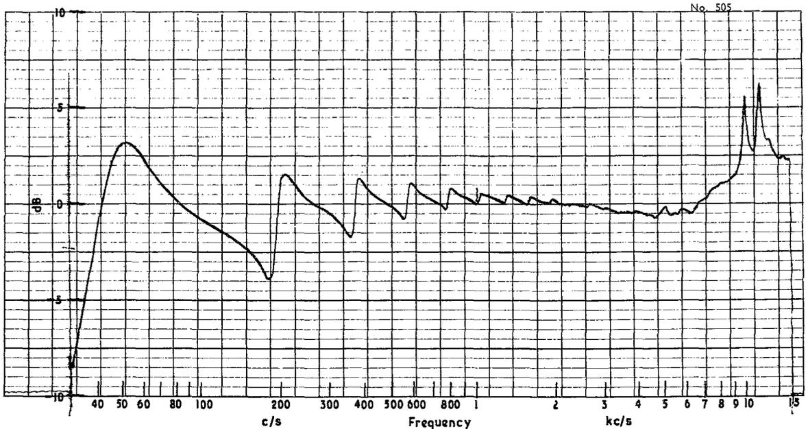
Fig. 3 - Example of curve taken with experimental ribbon using motional impedance bridge
