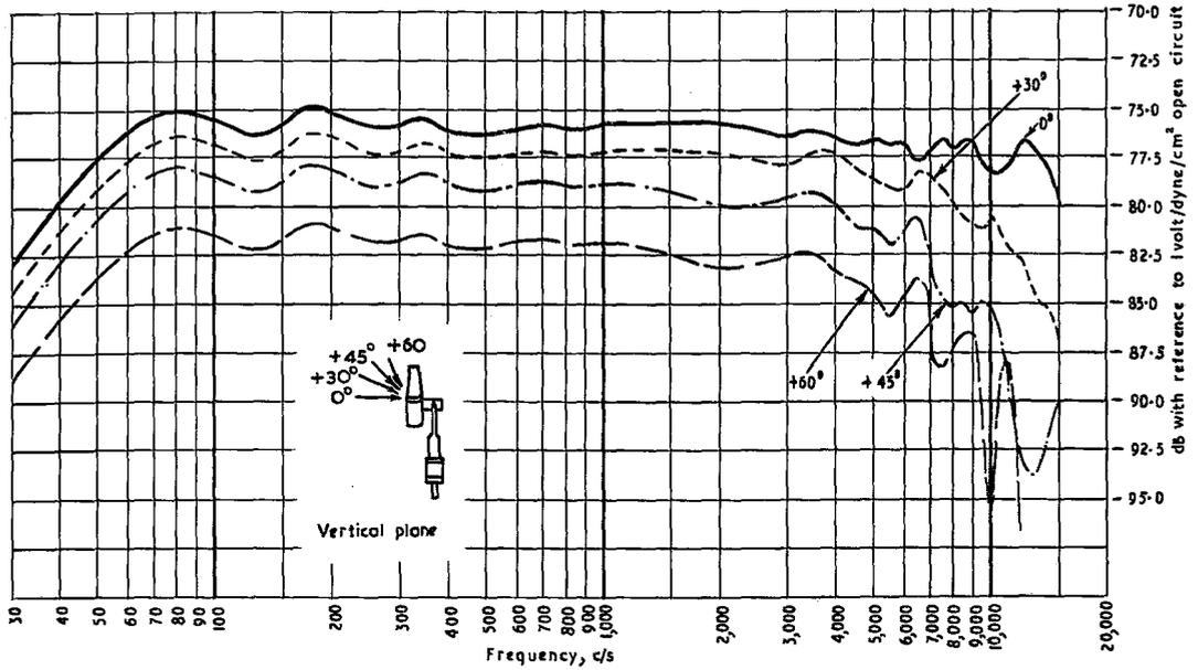
Fig. 7 - Microphone Type PGS. Open-circuit frequency response in vertical plane above axis
