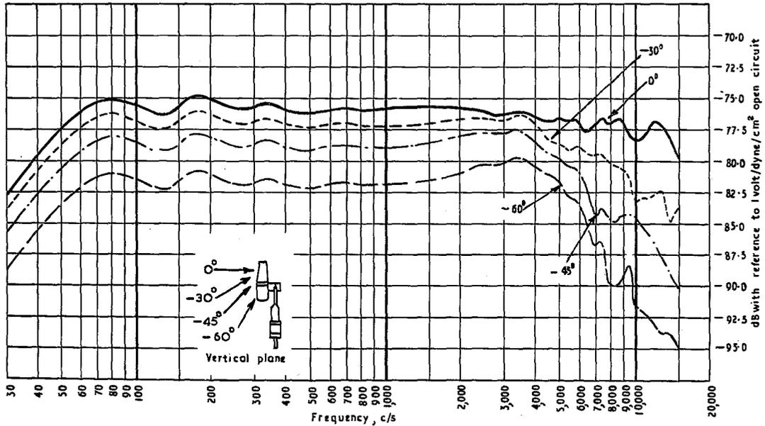
Fig. 8 - Microphone Type PGS. Open-circuit frequency response in vertical plane below axis
