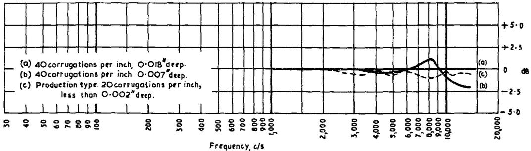
Fig. 2 - Microphone Type PGS. Change in high-frequency response with form of ribbon corrugation
