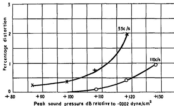
Fig. 12 - Microphone Type PGS. Total harmonic distortion
