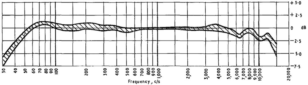
Fig. 9 - Production spread in axial open-circuit frequency response for PGS microphones
