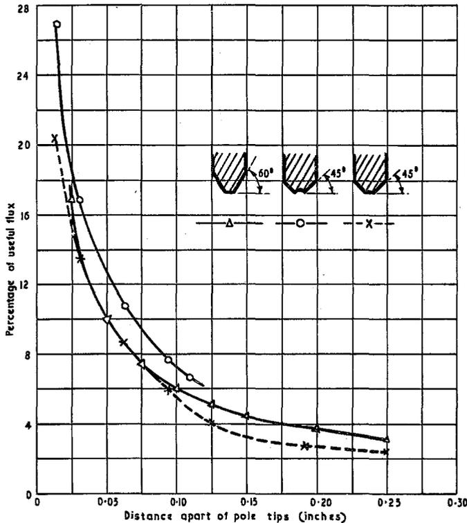
Fig. 1 - Microphone Type PGS. Ratio of useful flux to total flux between pole pieces. Data obtained by electrostatic model!
