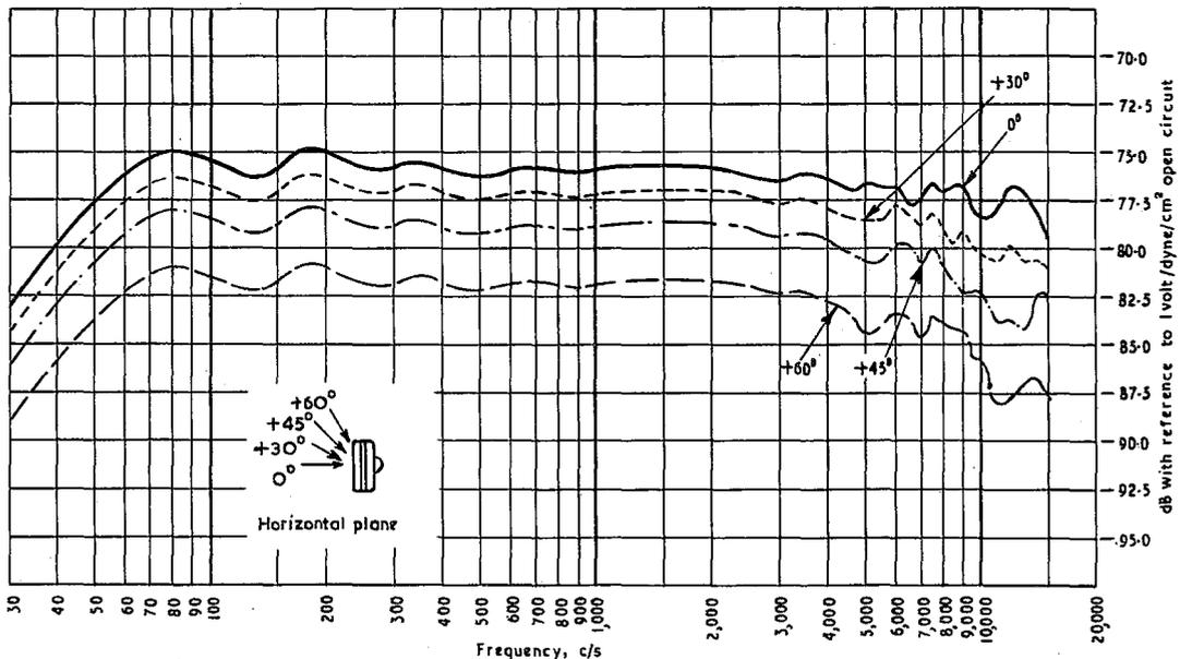
Fig. 6 - Microphone Type PGS. Open-circuit frequency response in horizontal plane
